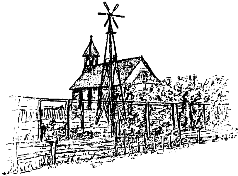
FIG. 73. The reconstructed Aermotor—a veritable toy—which cost nothing yet pumped water for the house, four head of horses, lawn, garden, and small fruit. By measurement it pumped, in a 15½-mile wind, 270 gallons in an hour, or at the rate of 6480 gallons in twenty-four hours; that is $1 worth of water in a day according to the rate of .0015 cents a gallon, as charged in Lincoln. Wheel eight feet in diameter. Depth of well twelve feet. Property of A. C. Walker, civil engineer.
