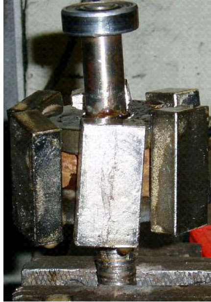
Figure 1. 40 amp car alternator rotor with magnets attached
