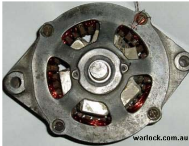
Figure 4. Completed conversion of the 40 amp car alternator
