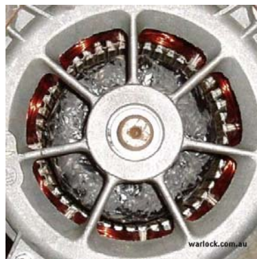
Figure 5. Completed conversion a ¼ hp induction motor
