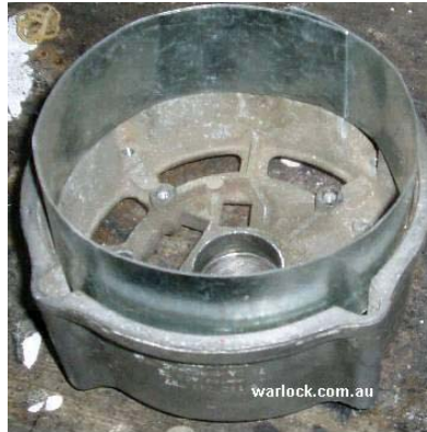
Figure 3. 40 amp car alternator stator with shielding
