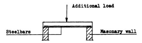
Due to dead load and additional loads such as people, earthfill, snow etc. the slab will get tensile stresses at the bottom. So in this place we must put some steelbars into the concrete.
