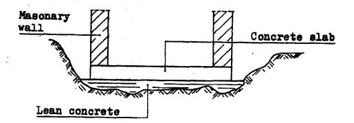
II. <u>Non-reinforced concrete</u>: To make foundations, floors small staircases, walls etc. All concrete constructions which are not exposed to high tensile stresses.
