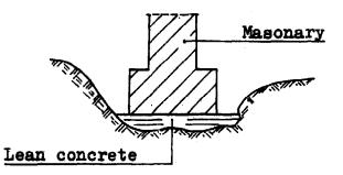
2. <u>Example</u>: Foundation of a spring collection chamber.
