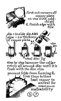
Making the plunger valve is a little more complicated, but it is somewhat simplified if we keep in mind that none of its parts needs to be machine-accurate. If there is some leakage through backflow of the water it will prove to be insignificant. Up-and-down pumping will open the bottom valve at each stroke and add more water to the column above it, filling the holding tank on top in no time while the bottom valve easily holds it there without leaking.
