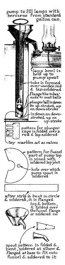
It must be remembered that each person wishing to make such a pump must do it from the odds and ends he has accumulated and that his supply is bound to differ from mine. The final appearance of his product, therefore, will probably be quite unlike the one I am showing here.
