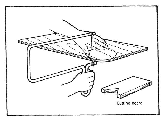
The fret saw is quite a specialized tool, not often used in carpentry workshops, but it is ideal for making childrens' toys and jig saw puzzles. The blade is very fine and is able to cut intricate shapes in thin timber and plywood, but it may be difficult to obtain. Unlike the coping saw, the blade cannot be adjusted, but this is overcome by the depth of the frame.
