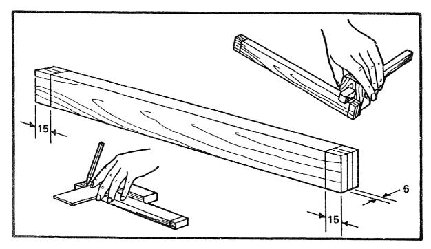
Take the crossbar and mark the shoulders of the tenons by squaring lines all round 15mm from both ends. With a mortise gauge, gauge a 6mm tenon on both ends of the crossbar.
