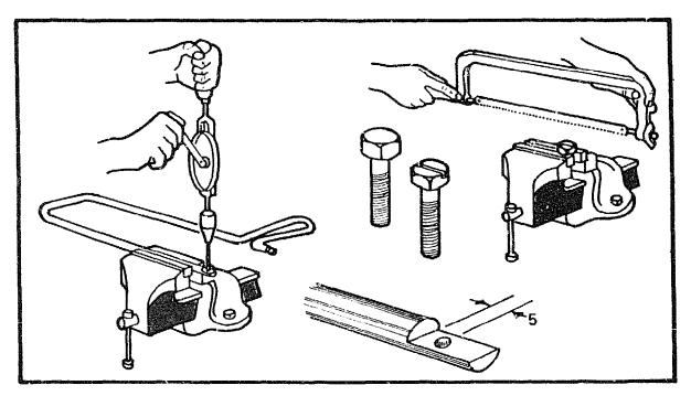
Punch and drill 6mm holes in the end of each leg of the frame. The centre of the holes should be exactly 5mm from the shoulder.
