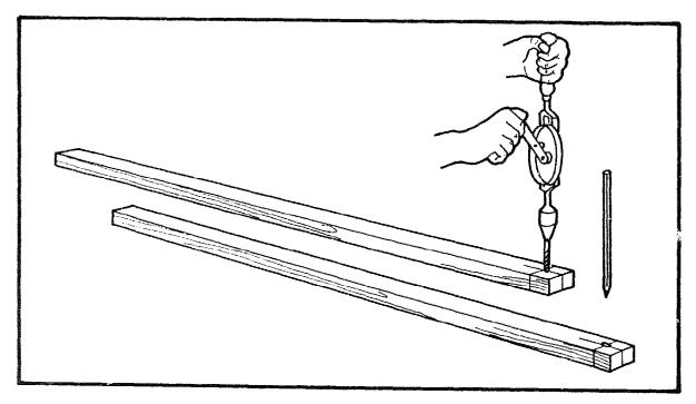
Drill a  $\emptyset$ 8mm hole from both sides of the stem. Fit a pencil into the hole
