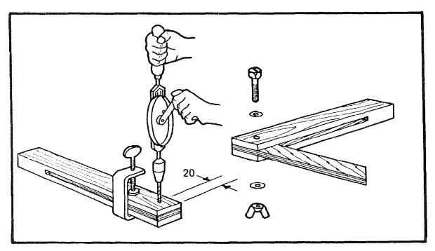
Fit the straight edge into the socket so there are no overlaps. Mark a central point 20mm from the end of the stock and drill a 6mm hole right through both pieces of wood.
