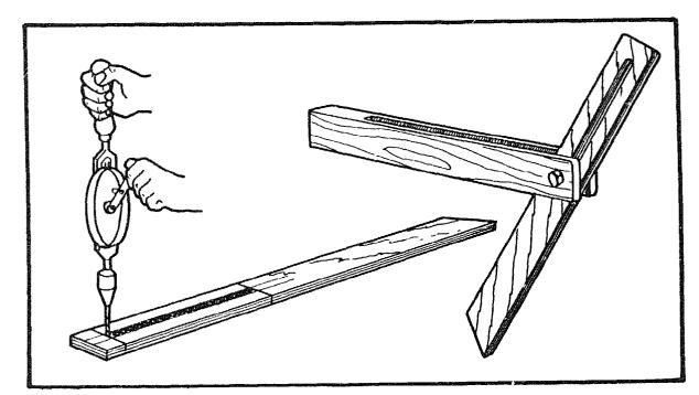
Drill a series of  $\emptyset$ 5mm holes between the gauge lines, clean out the waste with a chisel and file the slot smooth. Assemble the bevel square in the same way as shown on page 17.
