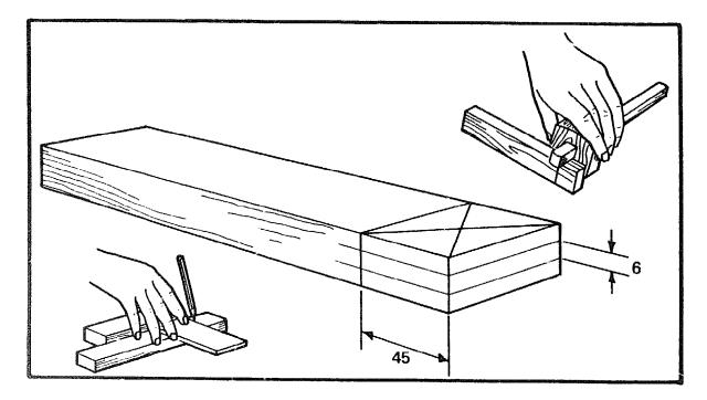
Take the timber prepared for the slock and square a line all round 45mm from one end. Gauge two lines 6mm apart in the centre of the stock. Draw diagonals to find the centre of the joint.
