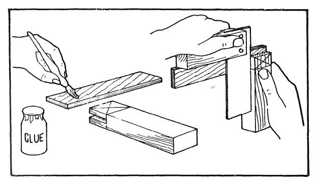
Glue the blade into the stock and, before the glue dries, make sure the blade and stock are square. Leave the assembly to dry.
