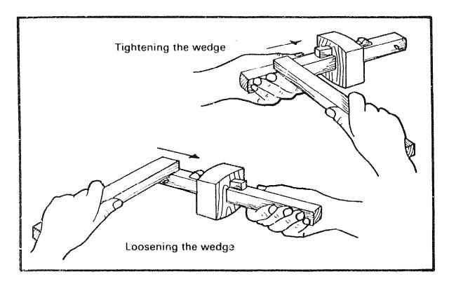
To use the gauge first set the distance from the spur to the fence. Tighten the fence to the stem by tapping the back of the wedge with a piece of wood. Check the setting and make final adjustments by tapping either end of the stem on the bench top.
