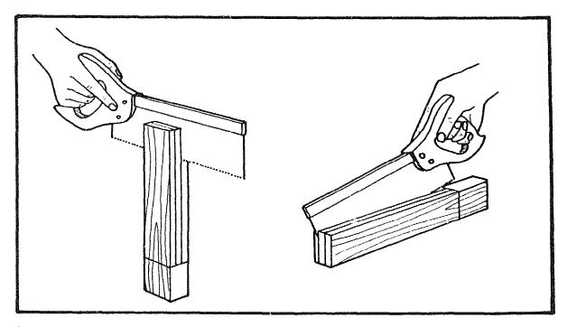
Use a tenon saw to saw out as much of the socket as possible.
