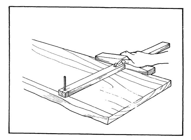
This is a large wooden gauge with a wide fence and a stem anything up to a metre long. Instead of the workpiece being marked with a metal spur, the stem carries a pencil, located in a hole at one end. The fence and the stem are locked together by a wedge.
