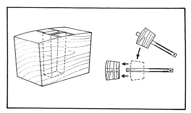
Shape the top of the mallet with a slight curve using a plane. The dotted lines in the drawing show the tapered mortise in the head. If the handle and the mortise was straight the head would soon fly off.
