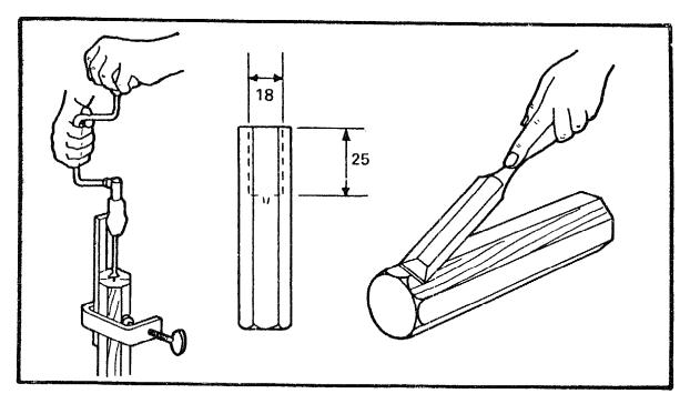
Where the diagonals meet, drill an  $\emptyset$ 18mm hole to a depth of 25mm.
