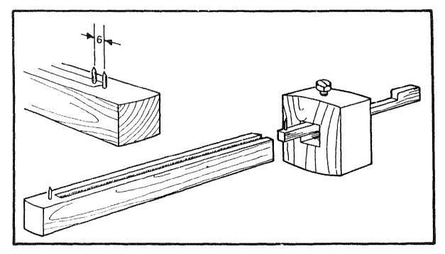
Fit the slider into the groove, so that the distance between the two spurs is 5mm. Sharpen the spurs with a file, and assemble the gauge.
