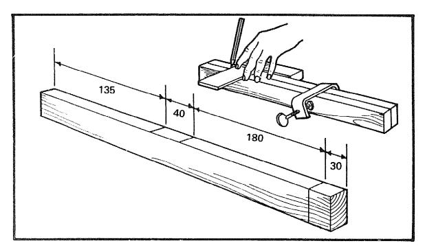
Clamp the two side frames together and square two lines across, 40mm apart, for the mortise. Square one line across, 30mm from the bottom, to mark the hole for the blade socket. Square this line all round both frames.
