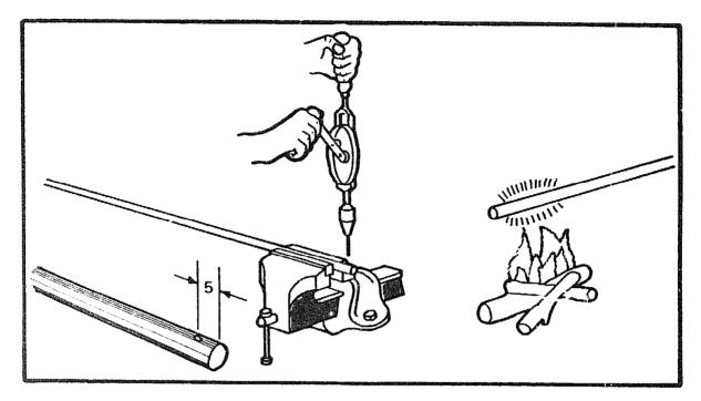
Centre punch and drill a  $\emptyset$ 3mm hole in one end of the steel rod (the hole should be slightly bigger than the nails to be used as blade holders). Build a fire from wood or charcoal. The frame can be bent easily if the rod is red hot.
