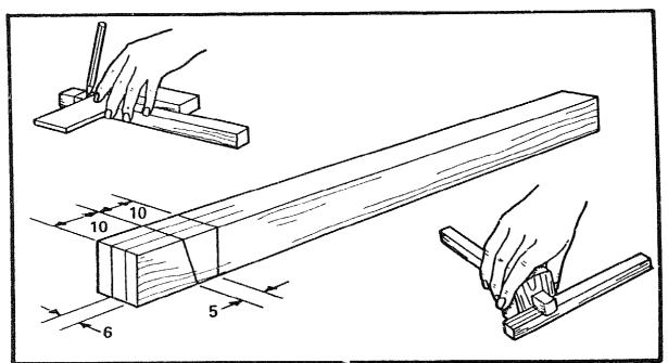
Take the timber prepared for the stem and square a line all round 20mm from the end. On the top square a line 10mm from the first line towards the end, and on the bottom 5mm from the first towards the end. When joined these lines mark the slope for the wedge. With a mortise gauge, gauge two lines in the centre 6mm apart to mark the mortise.
