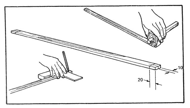
Take the timber prepared for the bow and square a line 20mm from both ends. Gauge a line in the centre of both ends to mark the holes for the bow string.
