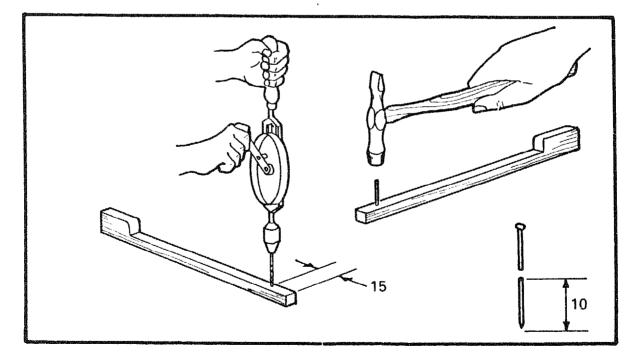
Use the same drill to bore a hole in the slider, 10mm from the end. Take another 25mm nail and cut it down to 10mm in length. Carefully hammer this into the slider, again leaving 5mm sticking out. Drilling the hole first should prevent the timber splitting.
