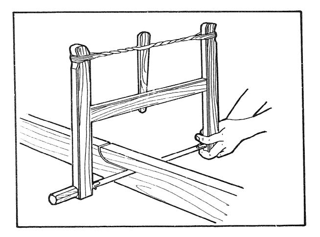
The bow saw is a difficult tool to make, involving metal work and wood work. Its advantage over the other types of saw in this manual is that the blades can be made from hack saw blades which are easily obtainable in most countries. This is not the case with fret saw and coping saw blades.
