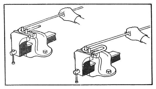
Make a 'U' shaped bending bar as shown on page 91. Heat the rod up and make the first bend 100mm from the end with the slit in. Heat the rod and make a second 180 degree bend opposite the end of the bar.
