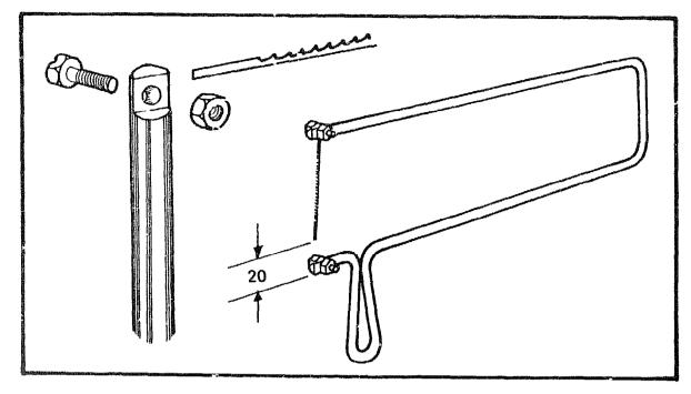
Place the bolts through from the round side of the frame and screw the nut on. The nut should not be able to turn because of the shoulder cut in the frame. Clamp the blade into one leg of the frame.
