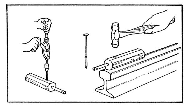
Push the 9mm bars into the handles, with the slot and the hole pointing out. 25mm in from the drilled end of the handle, drill a  $\emptyset$ 3mm hole right through. Push a 50mm (2") nail through this hole. Cut the end off and rivet the cut end of it with a hammer to hold the two pieces firmly together.
