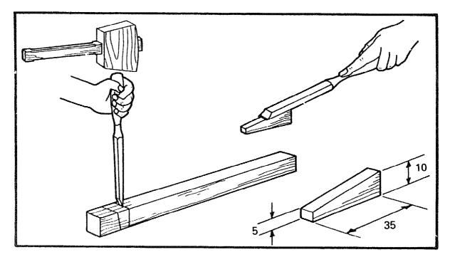
Cut the mortise between the pencil lines leaving a slope for the wedge. Make sure the ends of the mortise are straight.
