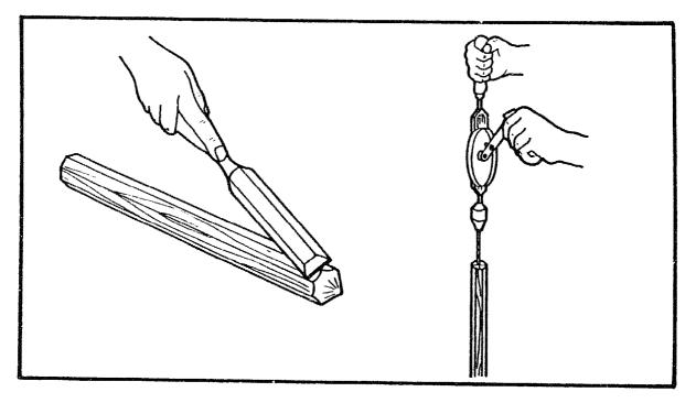
With a chisel or a sharp knife shape one end to a point. The tip of the point should be where the diagonals meet.
