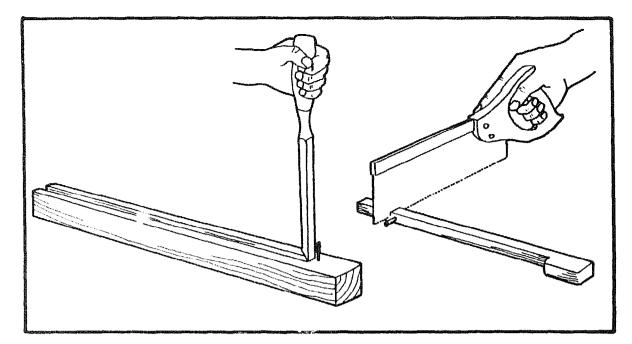
With a 6mm chisel, cut the groove back to within 3mm of the spur in the stem.
