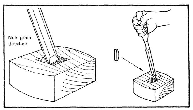
Make the fence as shown on pages 22 and 23, but do not cut the groove for the wedge. Instead carefully cut a recess in the centre of the mortise by first cutting the end grain with a chisel held at an angle. Then, with a 6mm chisel remove the waste.
