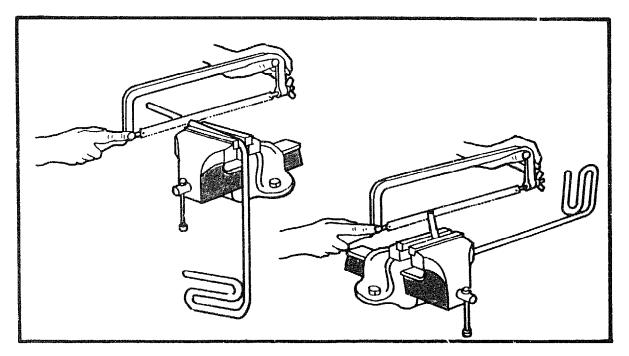
Measure and cut the front leg of the frame to the same length as the leg at the handle. Saw a slot down the middle of the front leg 12mm long with a hack saw.
