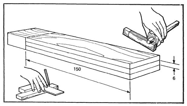
Take the timber prepared for the stock and square a line round 150mm from one end.
