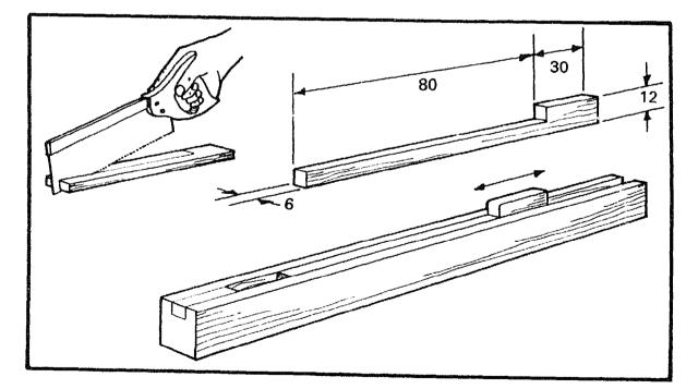
Cut the slider to the dimensions shown. Fit it into the groove. It should slide easily, but not wobble in the groove. The top of the slider can be scraped with a chisel so it is flush with the top of the stem.
