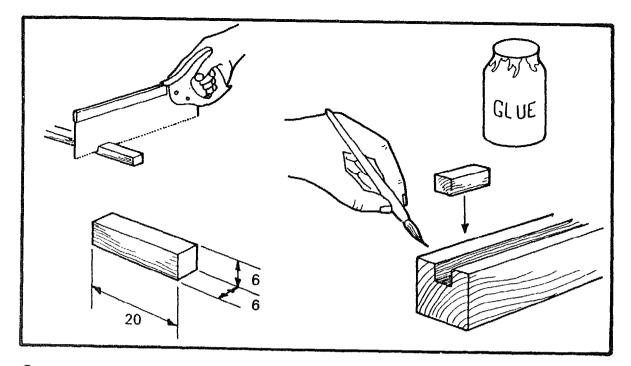
Cut a small block of wood from the piece prepared for the slider, 20mm  $\times$  6mm  $\times$  6mm. Fit and glue it into the groove at the end of the stem.
