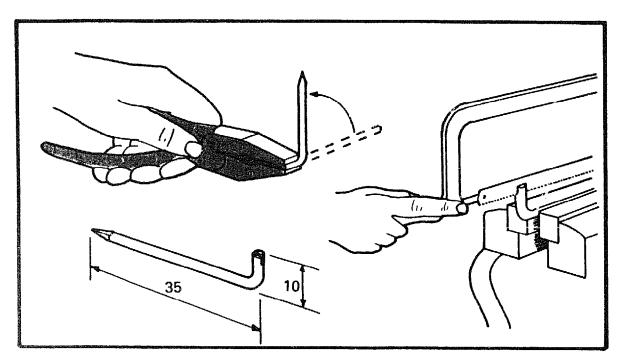
Saw the head off a 50mm nail leaving it 45mm long. Make a 90 degree bend 10mm from the sawn end. With a hack-saw carefully cut a slot about 4mm long down the centre of the nail.
