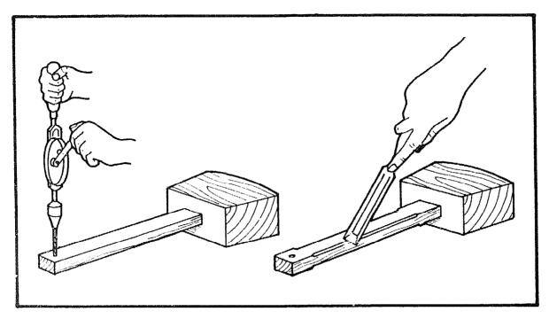
Drill a  $\emptyset$ 9mm hole in the end of the handle; this can be useful when storing the tool.
