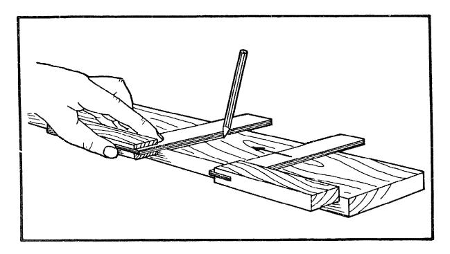
Take a piece of wood about 200mm wide, with face side and face edge planed straight and square. Place the try square on the timber and draw a line from the face edge. Turn the try square over to approach the line from the other side. If the square is true the pencil line and the straight edge will be parallel to each other.
