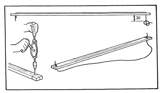
Drill two  $\emptyset$ 3mm diameter holes, one at each end of the bow. Thread the string through one hole and tie a knot. Thread the other end of the string through the other hole, and tie a knot 30mm from the hole.
