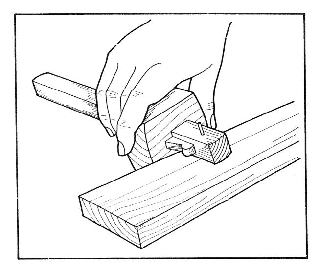
Marking gauges consist of two main parts, a fence and a stem. The stem carries a pointed metal spur at one end. The fence can be fixed to any position along the stem by a wedge as described here, or by a locking screw as shown on page 27 and page 41.
