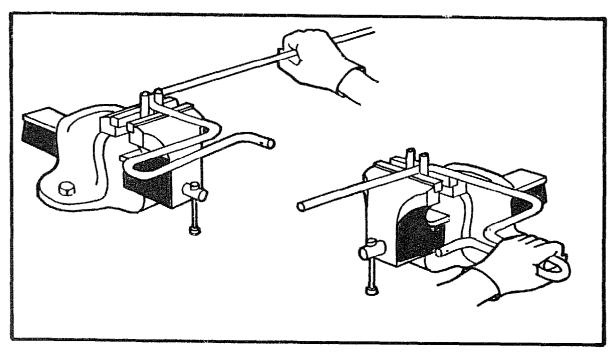
Measure 140mm from the end of the rod, heat it up until red hot, and make another 90 degree bend.
