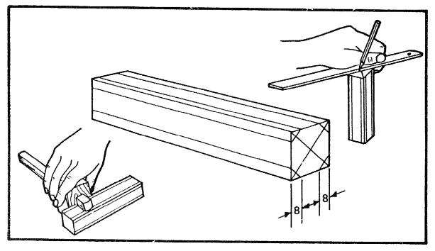
Take the timber prepared for the handle, and gauge eight lines 8mm in from each edge.
