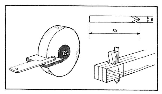
Grind a small piece of hacksaw blade to the dimensions shown, with a 'V' shaped bevel on the end. If you do not have a grinding wheel it can be filed, but first it must be heated until it is red hot, to soften the steel.
