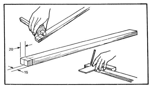
Take the Umber prepared for the stem and square a line all round 20mm from the end. On top and bottom, gauge a centre line which should be 15mm from both sides.
