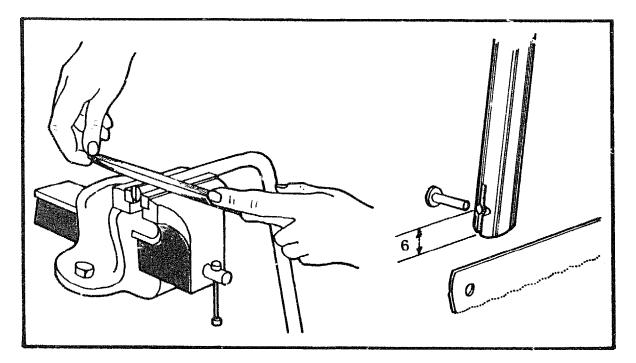
File a small nick, 6mm from the end of each leg, on the outside of the frame. This helps secure the blade holder. The blade holder is made from two cutdown 50mm nails.
