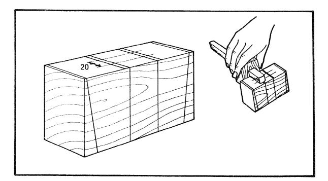
On the top and bottom of the head gauge two lines 20mm apart in the centre, with a mortise gauge.
