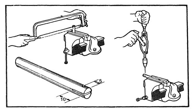
Take the two pieces of 9mm bar and saw a slot 10mm long in one end. 5mm in from the same end, punch and drill a  $\emptyset$ 3mm hole right through.
