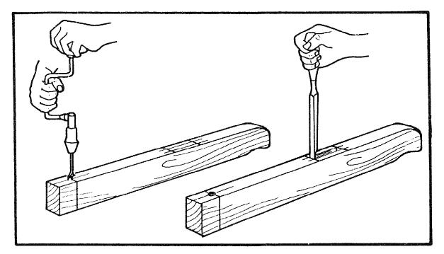
From both sides, drill a  $\emptyset$ 9mm hole, with a brace and bit. With a 6mm mortise chisel and a mallet, cut the mortise to a depth of 20mm.
