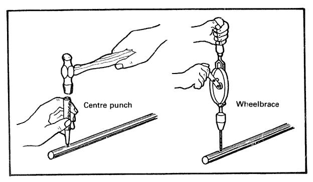
*Drilling a hole.* It is important to punch a small dent in the workpiece first. This will keep the drill bit from wandering off the mark.
