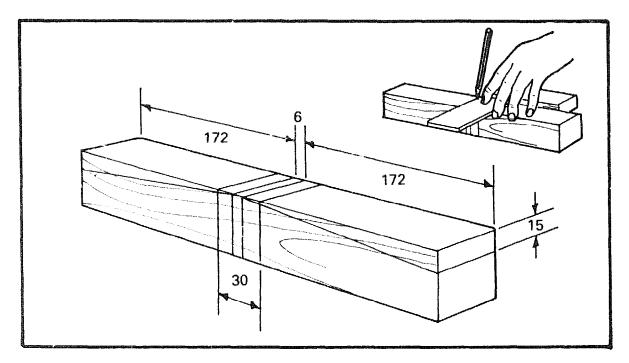
Take the timber prepared for the fence, mark a point in the centre, and square two lines all round 3mm either side. Square two lines all round 15mm either side of the centre mark. On each end, square two lines 15mm below the top edge.
