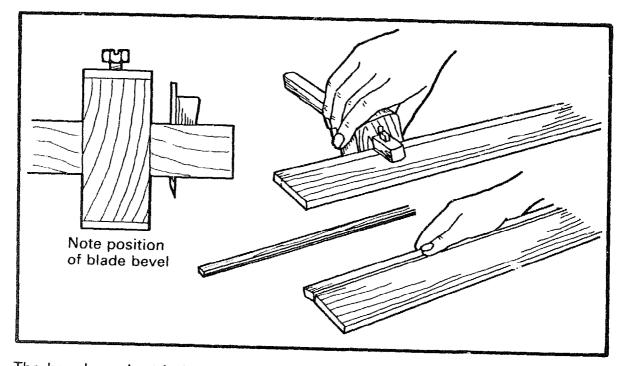
The bevel on the blade should face the fence, otherwise it will follow the grain. Cutting gauges can be used for cutting thin strips of wood for making small beadings or dowels. Score the timber on both sides and break the piece off with your hands.
