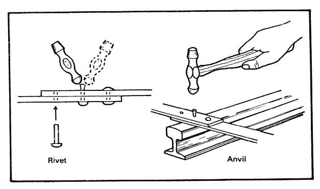
*Riveting.* This technique can be used to fix two pieces of metal, or sometimes a combination of wood and metal, together. Rivets can be bought or made from nails. They should be about 5mm longer than the thickness of the joint. Push the rivet through the hole, and spread the end by hitting it at differing angles round the head with a ball pein hammer.
