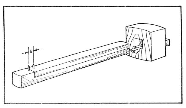
Fit the two parts of the stem together and if necessary trim the ends with a chisel or sharp knife so that the distance between the spurs is 6mm. Mark and cut the back end of stem C so that it is flush with the end of stem A and assemble the gauge.
