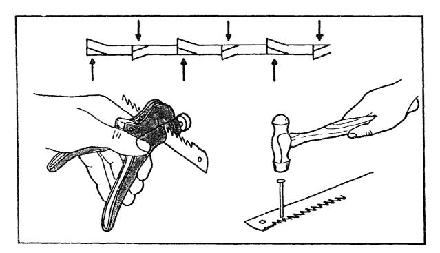
The teeth of the blade now have to be set. Use a saw set if one is available. If not a hammer and a blunt nail can be used to bend the first tooth to the left, the next to the right, and so on.
