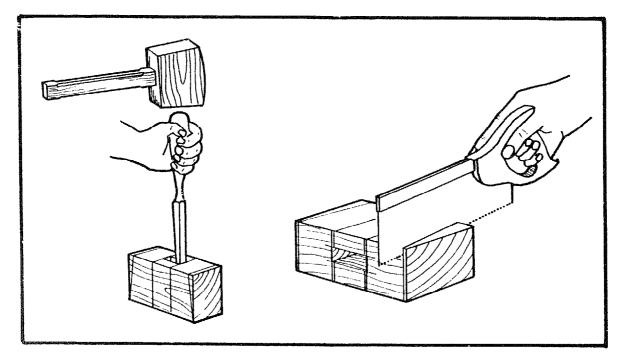
Cut the mortise with a mallet and chisel. Note how, at 34mm, the mortise is 4mm bigger at the top than the bottom. With a tenon saw cut the angled ends of the mallet head.
