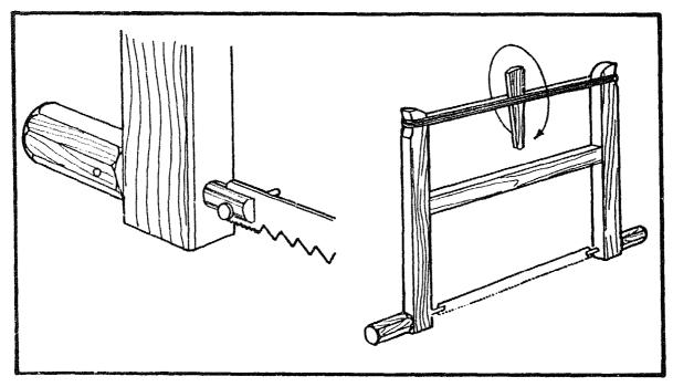
Now assemble the three parts of the frame. Push the blade sockets through the holes in the side frames and attach the blades with two 50mm nails cut down to about 20mm long. Wind some string three or four times around the top of the frame and tie the ends together. Slip the twisting slat through the string and twist it until the blade is tight, then slide it down until it rests on the crossbar.
