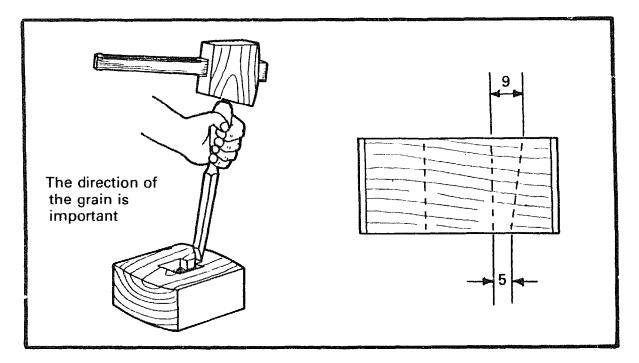
With a 6mm chisel and a mallet cut a sloping groove into the mortise of the fence. It should run from about 9mm at the big end to about 5mm at the small end.
