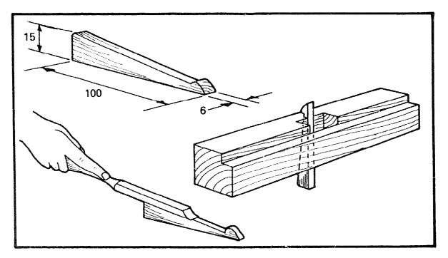
Cut the wedge to the dimensions shown, with a small knob at the end. This will stop the wedge falling out. Shape it so that it fits properly into the groove in the fence.
