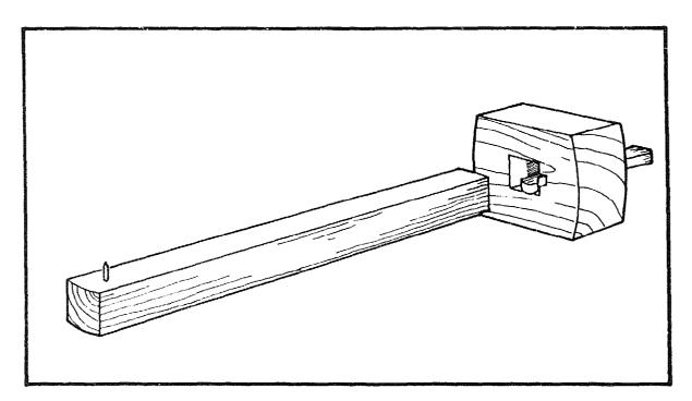
Assemble the marking gauge by fitting the wedge into its groove and sliding the stem through the fence. If it does not fit check that the sides of the mortise are straight, or plane the stem down very carefully.
