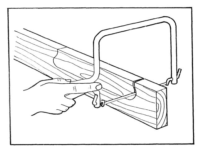
The coping saw is a small version of the bow saw. It has a very narrow blade, held in tension by the spring of a steel frame. The blades have to be replaced when they become blunt and must be bought from a shop.
