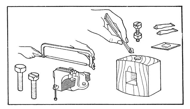
Take the 20mm  $\times$  6mm nut and bolt and saw a slot into the head for a screwdriver.
