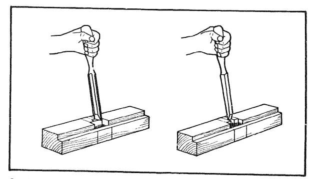
Carefully cut the groove for the wedge. First cut across the end grain on both sides with a mallet and chisel. Second, remove the waste with a 6mm chisel.
