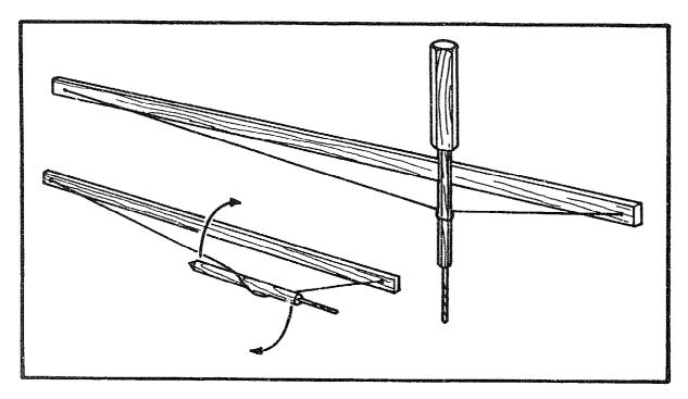
Twist the bow string once around the stock of the drill. Put some grease or cooking fat on the point, and push it into the hole in the handle.
