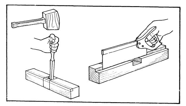
Chisel out the mortise. Cut the rebate with either a tenon saw, or a rebate plane.
