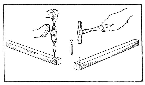
From both sides drill a hole with a bit slightly smaller than the diameter of the nail you will use as the spur. If you do not have a bit small enough, cut the head off a 20mm nail and use this to make the hole.
