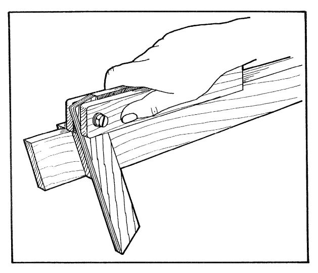
A bevel square, which is an essential tool for marking out dovetails and other joints with angles greater or smaller than 90 degrees, can be made on the same lines as the try square. Again the dimensions given are only for guidance.
