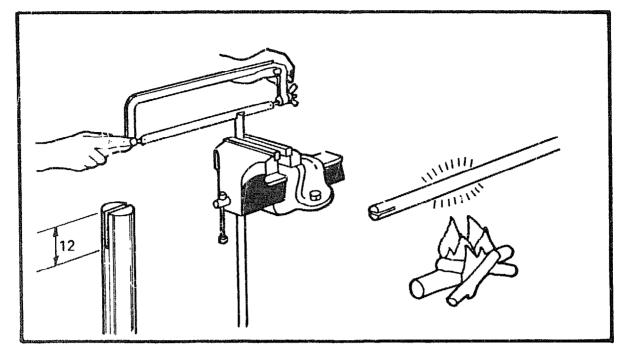
Take the rod and cut a slit down the centre, 12mm long, in one end with a hack saw.
