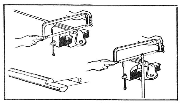
Take the rod and saw out a semi-circular section 12mm long, using a hack saw.
