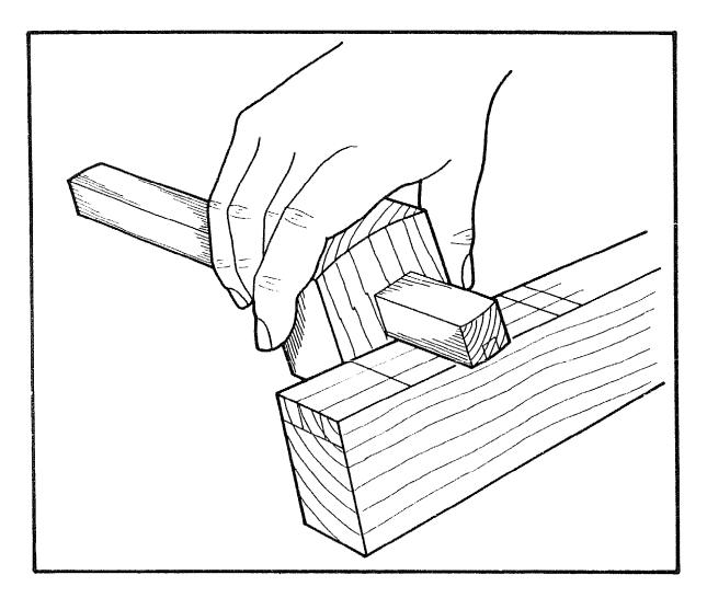
This design is based on the mortise gauges available in most tool shops. It is easy to use, but requires a higher degree of skill to construct.
