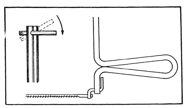
When using the coping saw make sure the blade is not twisted and the teeth point towards the handle. The blades are not strong so use the saw carefully.
