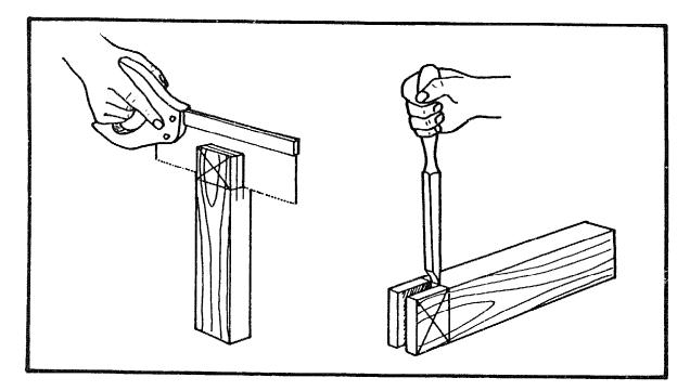
Saw out the socket with a tenon saw and chisel out the waste.
