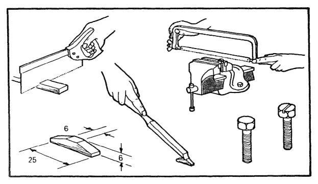
Take the timber prepared to make the wedge and the shoe and cut a small piece off  $25mm \times 6mm \times 6mm$ . Shape the shoe as shown with a chisel. Take the  $20mm \times 6mm$  bolt and saw a slot in the head for a screwdriver.
