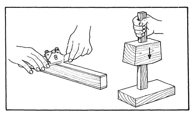
Shape the handle with a spokeshave or a plane down to the lines. To fit it, push the bottom of the handle through the top of the head and tap it down on a piece of wood.
