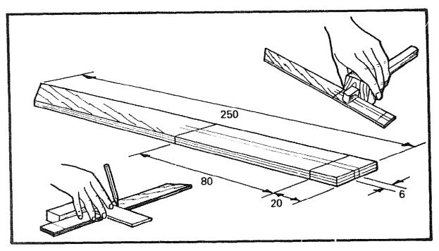
Prepare a piece of 6mm plywood 250mm  $\times$  40mm. Square a line 20mm from one end and another 100mm from the same end. Gauge a 6mm slot in the middle of the plywood between the two lines. Cut a 45 degree angle off the other end.
