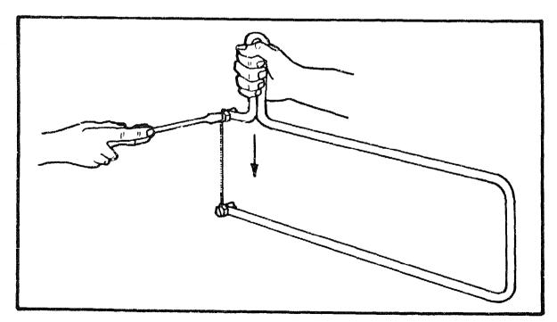
Push the frame together and fix the blade at the back (between the nut and the flat part of the frame).
