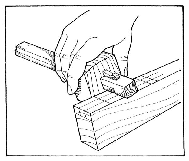
Mortise gauges are made with two spurs which mark two lines parallel to the edge of a workpiece, showing the position of a tenon or mortise or a similar joint. This avoids having to score two lines spearately, and makes for greater accuracy. The spurs must be able to move independently, and be locked in any position by the fence. This makes it quite a difficult tool to construct.
