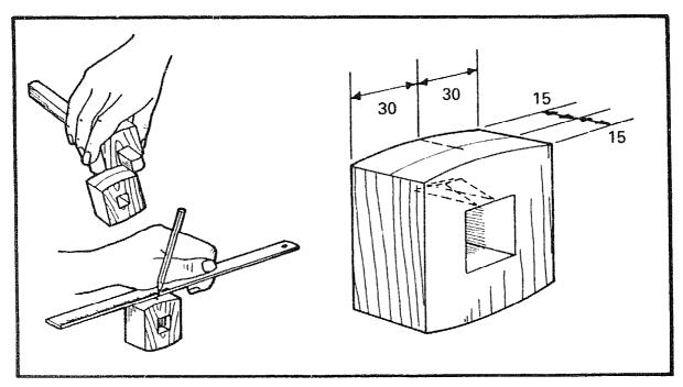
To make the fence follow the directions on pages 22 and 23, but do not cut the groove for the wedge. Instead choose one edge of the fence with end grain and gauge a centre line, which should be 15mm from each side.
