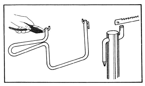
Push the sharp end of the nail through the hole and bend it 90 degrees in the same plane as the first bend. Do this at both ends of the frame.
