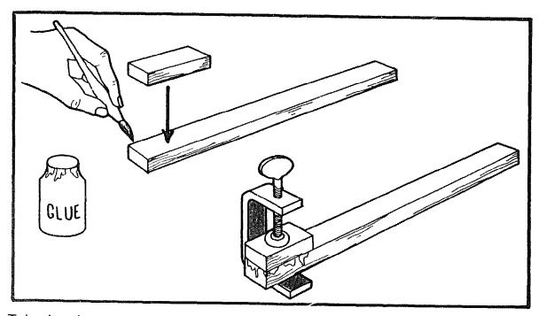
Take the pieces prepared to 200mm  $\times$  10mm  $\times$  20mm and 30mm  $\times$  10mm  $\times$  20mm. Glue and clamp the smaller one to the end of the larger one, and make sure there are no overhangs. Plane the glue off when it is dry.
