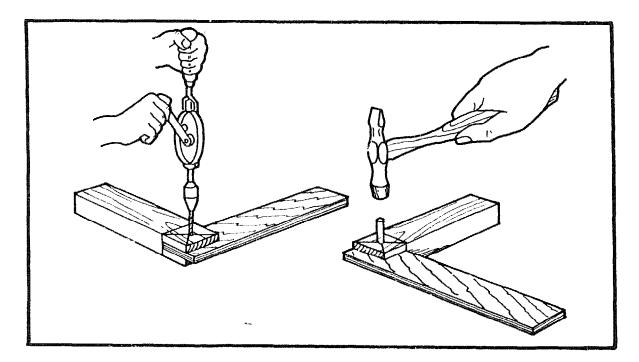
When the glue is dry drill a  $\emptyset$ 6mm hole in the centre of the joint. Drive in a 6mm dowel. Plane the back of the blade flush with the stock and smooth up the ends of the dowel.
