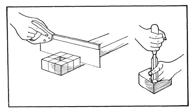
Saw the fence off on the pencil line 60mm from the end. You can round off the corners with a plane or chisel and smooth it with sandpaper.
