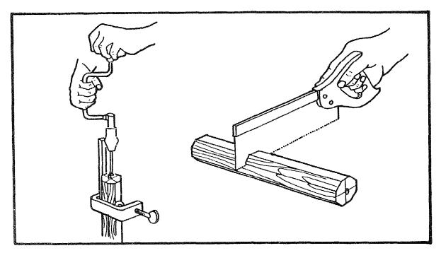
Drill a  $\emptyset$ 9mm hole in both ends, 50mm deep. Clamp a small piece of timber to the handle to help you to drill the hole straight. Saw the handle into two pieces, one 60mm long, the other 100mm long.
