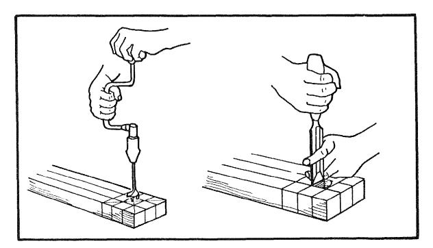
With a brace and bit, drill a  $\emptyset$ 20mm hole exactly where the diagonals meet. Drill half way through, then turn the timber over to drill from the other side. Square the hole up to the gauge and pencil lines with a chisel.
