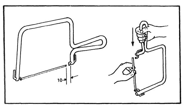
Bend the legs of the frame so that the gap between the two blade holders is 10-15mm bigger than the blade. This gives the right blade tension.
