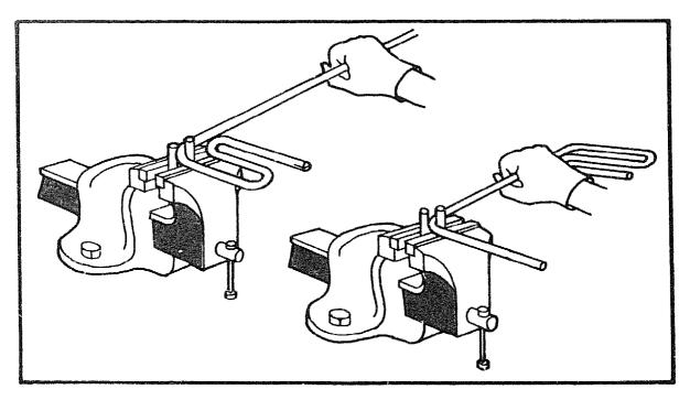
Heat the rod and make an 80 degree bend (see drawing of frame) so it just touches the first 180 degree bend. Heat the rod, measure 300m from the last bend and make one more 80 degree bend.
