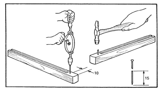
Take a 25mm (1") nail and cut it down to 15mm. Drill a hole slightly smaller than the diameter of the nail, 15mm from the end of the stem. If you do not have the right size bit, cut the head off a 20mm nail and use that to make the hole.
