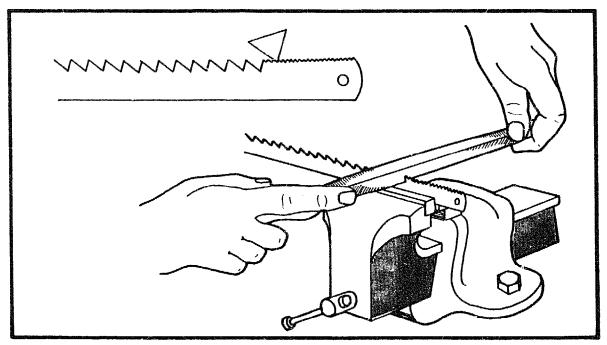
To make a blade for the Bow Saw, a hacksaw blade must be softened. Only the cheaper "low-speed" blades can be used. Put the blade into a fire until it is red hot. Take it out and let it cool down slowly beside the fire. With a saw file, file every third tooth until it is three times bigger. Take care to make each tooth the same size.
