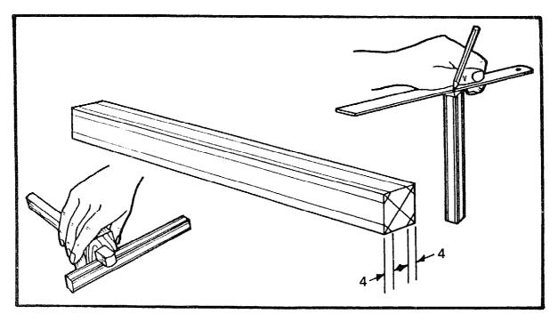
Take the timber prepared for the stock; find the centres of each end by marking the diagonals. Gauge eight lines, 4mm in from each end. Plane off the corners down to the gauge lines.
