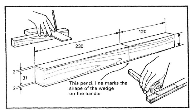
Square a line all round 120mm from the end of the handle. From this line gauge 2mm on both sides, to the other end. With a pencil mark the wedge shape at the top of the handle.
