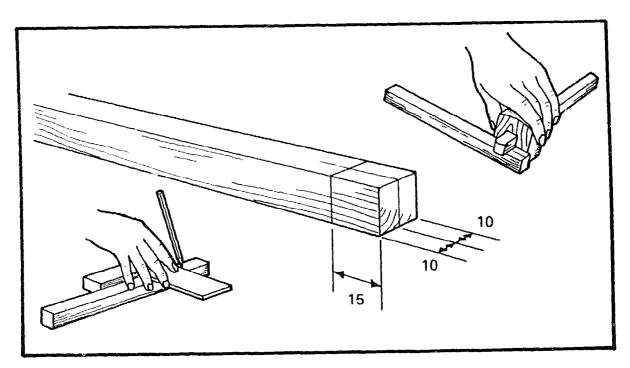
Take the timber prepared for the stem and square a line all round 15mm from the end. On two opposite sides of the stem gauge centre lines, crossing the pencil lines.
