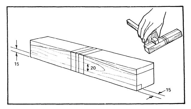
On one bottom edge gauge a 15mm  $\times$  15mm rebate. On the two sides gauge a line 35mm from the bottom edge, for the mortise.
