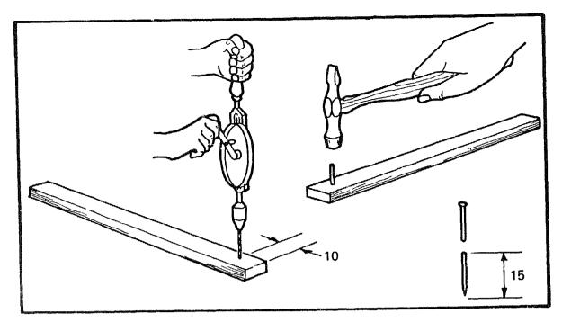
Take the timber prepared to  $180 \text{mm} \times 10 \text{mm} \times 20 \text{mm}$ , and using the same bit, drill a hole 10mm from the end of the timber. Cut a 25mm (1") nail down to 15mm.
