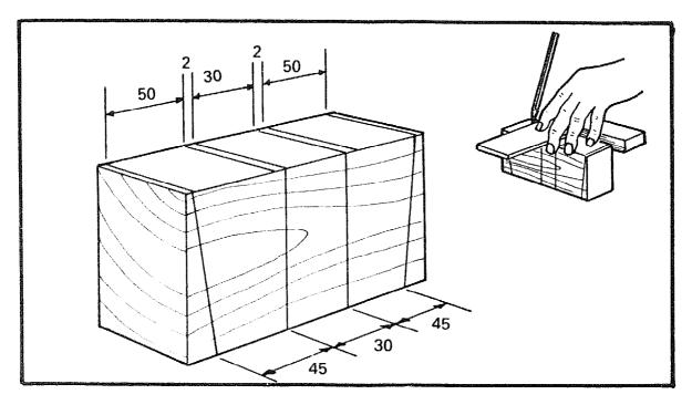
Square two lines 30mm apart in the centre of the block. On the top mark two lines 2mm towards the end. Now mark the angled ends of the mallet head, by squaring two lines 50mm towards each end, on the top, and two lines 45mm towards the end, on the bottom.
