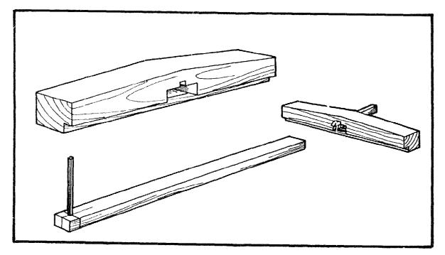
The fence can now be shaped by planing off the top down to the pencil lines on the end grain. This will make it a bit lighter.
