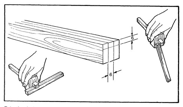
Take the timber prepared for the stem, and mark a 6mm groove down the centre of one side with a mortise gauge. Mark the depth at each end to 6mm.
