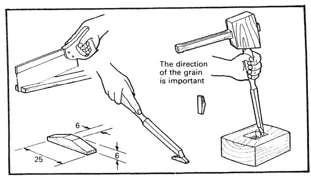
Cut and shape and the shoe from the timber prepared to  $200mm \times 12mm \times 6mm$ . With a mallet and 6mm chisel carefully cut a recess for the shoe in the end grain of the mortise, nearest the centre mark.
