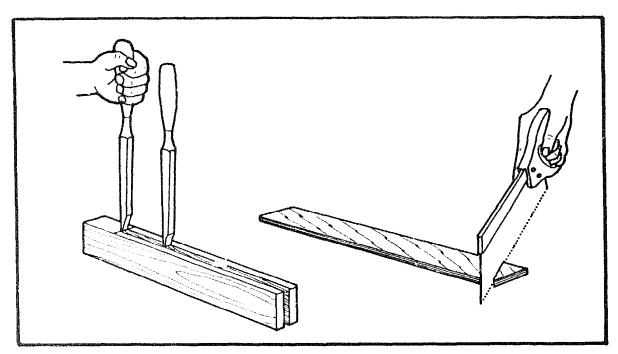
Use a 6mm chisel to cut out the waste wood in the stock. Take the plywood prepared for the straight edge and saw a 45 degree angle off one end.
