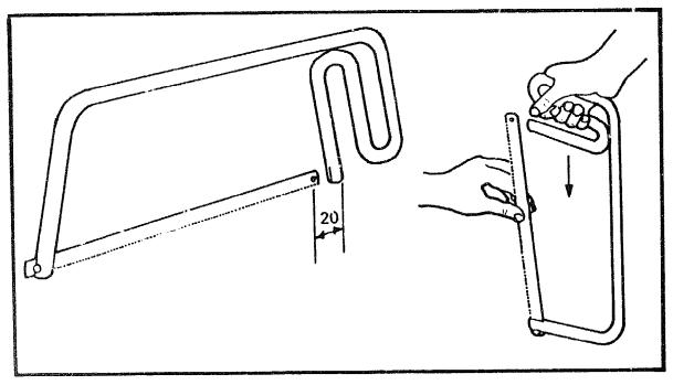
Bend the frame until the distance between the outside of the legs is 330mm. This gives the blade tension.
