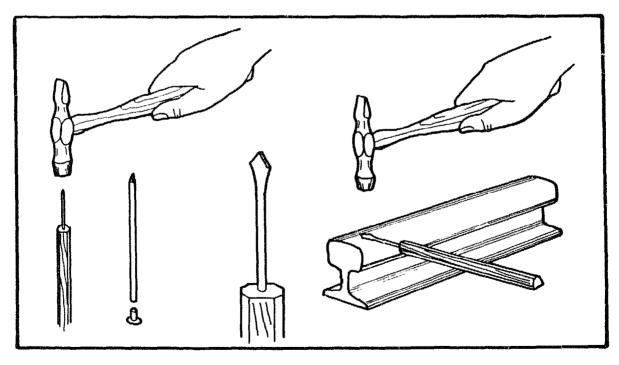
To make a wood-cutting bit from a nail. Take a suitably sized nail, cut the head off, and hammer the blunt end into the hole in the drill stock. Flatten the pointed end with a hammer on an anvil into a diamond shape. Sharpen the point with a file.
