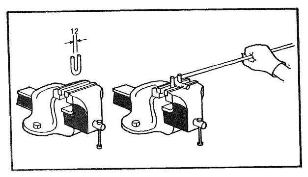
From a piece of 12mm rod make a 'U' shaped bending bar, with a 12mm gap between the uprights. Put this into a vice with about 20mm sticking out from the jaws. Heat up the end of the rod with the hole in and make a right angled bend 30mm from the end.
