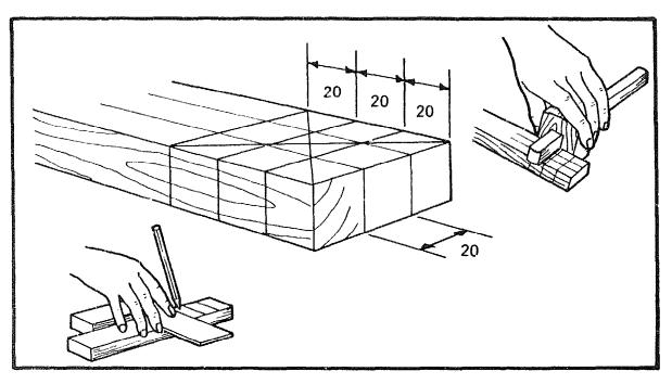
Take the timber prepared for the fence and square three pencil lines 20mm apart all round the timber; the first line should be 20mm from the end. Use a mortise gauge to mark two lines 20mm apart in the centre of the fence. Now mark the diagonals to find the centre of the mortise on both sides.
