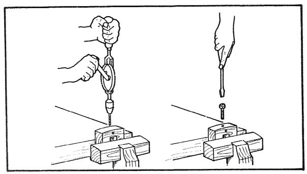
Mark the centre of the top of the fence, and drill a  $\emptyset$ 5mm pilot hole right through into the recess for the shoe. The pilot hole must not be drilled through the end grain.
