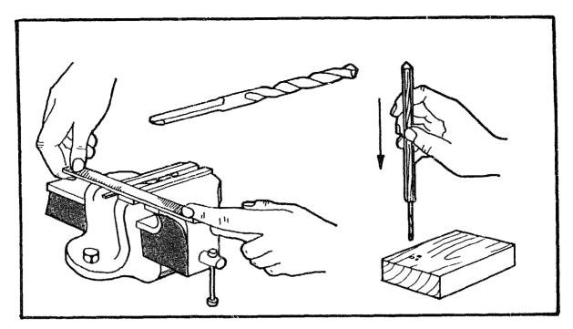
Take the drill bit and file two flats on the shank, and a point on the blunt end. Tap the bit into the stock, taking care not to blunt it. It may be necessary to use a hammer.
