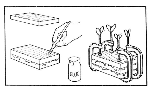
The mallet head can be made up of two or three pieces of timber, glued together. Make sure there are no gaps in the joints. Leave it clamped up for at least six hours.
