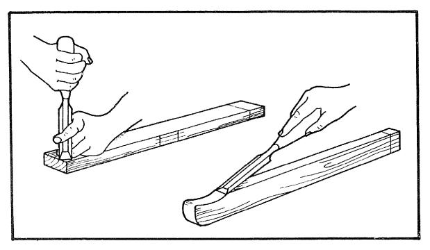
With a large chisel, shape the top of the side frames so that the string does not slip down. You can also round off the top inside corners.
