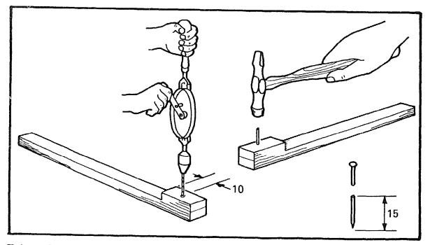
Take a 25mm (1") nail and cut off a piece 15mm long. Drill a hole, slightly smaller than the diameter of the nail. Use a small nail as a drill bit if you do not have one the right size.
