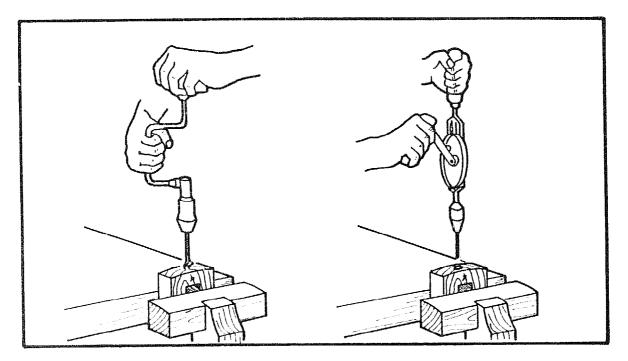
With a 12mm drill bit bore a hole on the centre mark to a depth of 6mm. Now drill a  $\emptyset$ 6mm hole right through, into the recess cut for the shoe.
