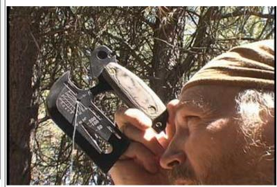
Just sight along the top of the blade and read the angle from the graphic. In the video we show you how to estimate the height of a tree or other object with the ATAX.
