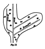
In fig. 12 is shown an adaptation of both systems to suit the land. Upon the right is a narrow piece of flat land, extending some distance from the main, which can be drained most economically by two parallel branches running at a proper angle to the main. At the left of the main is a flat extending lengthways of the main, but wider than can be drained by it, hence a small branch is laid out parallel to the main.
