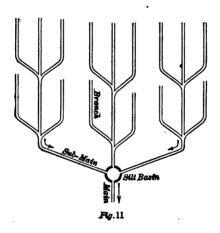
Again, mains must be made of larger tiles than any other of the lines, and so cost much more per foot. Crooks in the line increase its length and consequent expense.
