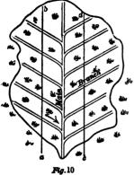
branch drains. The nearer the mains can be brought to these the less will be the expense of the branches and the more effectual will be their action. By these observations the farmer has an accurate method of finding the lowest places through which all main lines of drains should pass. The variation in the course of the main to suit particular
