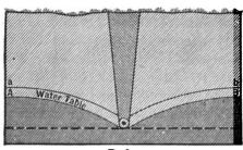
locity of flow is increased, but the depth of drained soil is decreased. The fact that the tiles are porous does not increase the flow nor add to their draining
