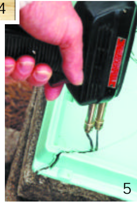
5. A flattened and hot soldering tip slices its way through plastic refrigerator shelves that are recycled into dam plates.
