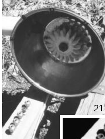
21. With the bowl removed, nozzle jets may be exchanged.
