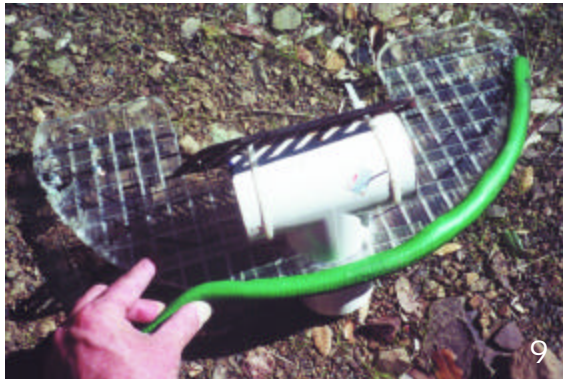
9. A split rubber hose acts as a gasket for the culvert dam.
