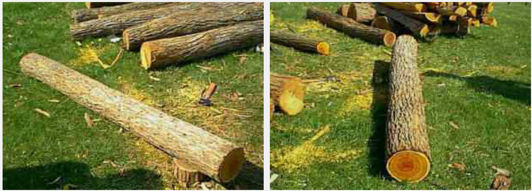
Examples of hard to find Osage Orange Stave material; Straight, No Knots, Limb Growth, or Twisted Trunk. Osage Orange likes to grow twisted with many limbs up the trunk. You can prune your crop of Osage Orange to get this result 25 years later.
