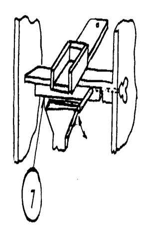
Stove bolt is 3/16" by 2". The winged nut is turned hard against the head of the bolt with epoxy against the head and in the threads. This makes a solid unit of the bolt and winged nut.
