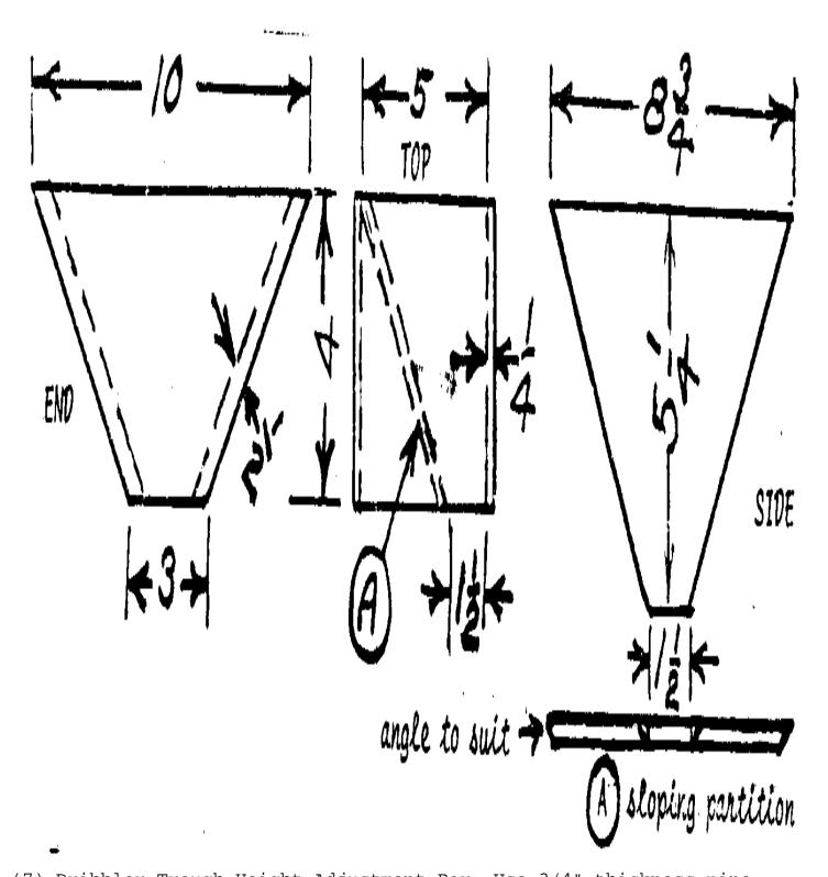
(7) Dribbler Trough Height Adjustment Bar. Use 3/4" thickness pine. hfm007.gif (437x600)
