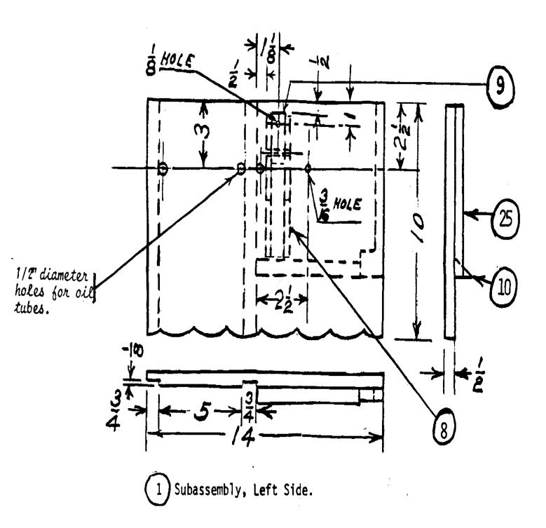
Use 1/2" thickness good quality plywood for parts (1) and (2) and 3/4" thickness
