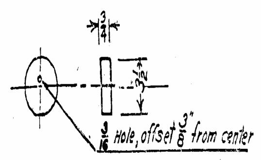
should be identical. Use epoxy under and around the head of the 3/16" bolt (inside mill body) on which these eccentrics turn. The one eccentric serves as a belt tightener and the other raises or lowers the grain hopper. Use winged nuts for convenience.
