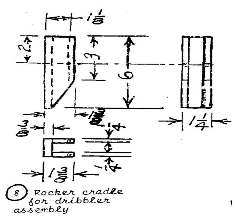
rocker bar, dribbler trough height adjustment bar and the revolving buhr holder are all shown digramatically in the sketch below. Notice that the eccentric action of the buhr holder provides the shaking action that causes the grain to work slowly to the end of the dribbler trough where it falls into the funnel shaped part #19 that directs it
