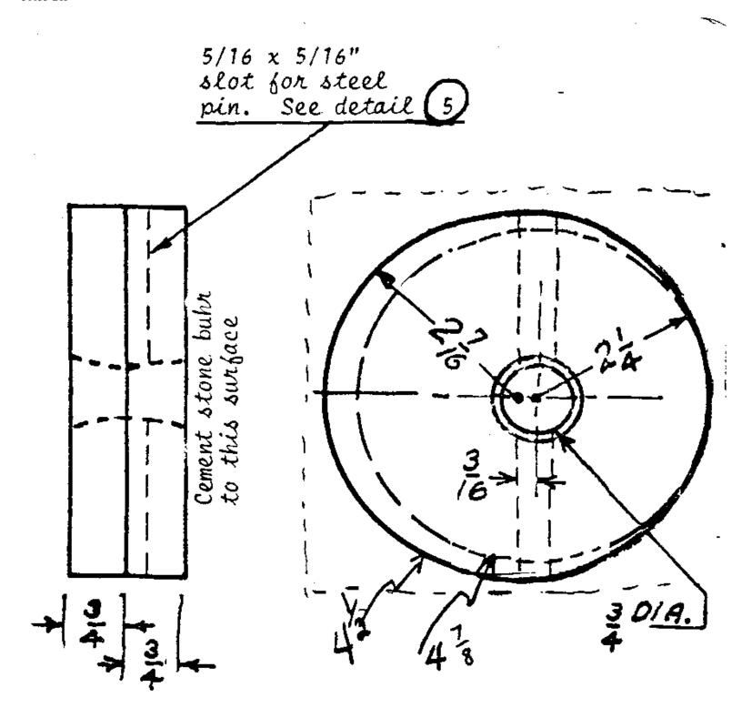
Use two pieces each 3/4" thickness plywood by 5" x 5". Before cutting the pieces round cut the 5/16" by 5/16" slot in one of the pieces as shown. Fasten the two pieces together using about four screws and glue. The 3/4 diameter hole should next be located. This hole should pass exactly thru the center of the 5/16 x 5/16" slot. Before boring
