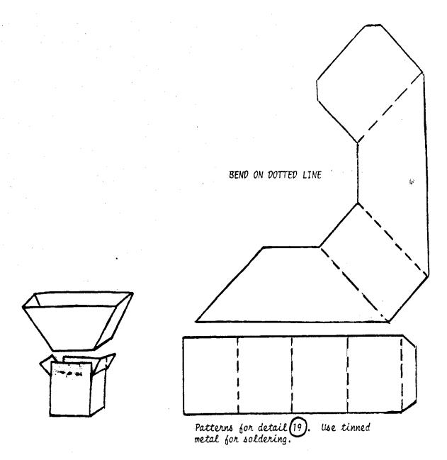
part. The auxiliary sketch shown here will help you. Use tin shears to make 1/4" cuts in each of the four corners of the square tube. Solder the seam of this tube then solder the seam of the rectangular funnel shaped section. Then, with two of the upper edges of the tube bent to conform with the funnel-shaped section, place the two parts together and solder.
