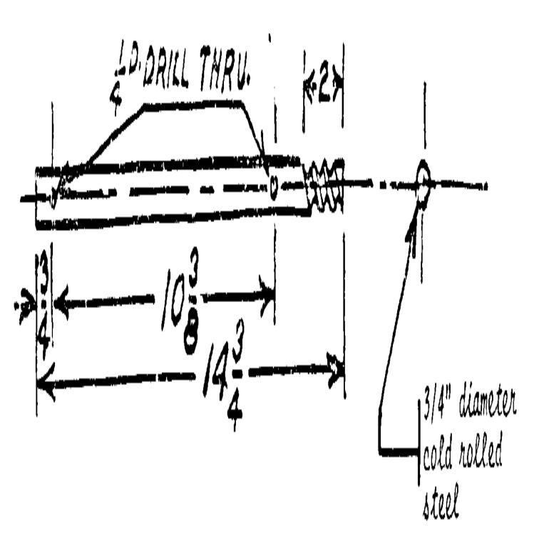
3/8 inch thickness grinding wheel or a 3/8 dia. round file to cut the spiral groove on one end. Cut the spiral groove about 5/32 of an inch deep. Follow drawing as closely as possible; however, some unevenness in the screw will not
