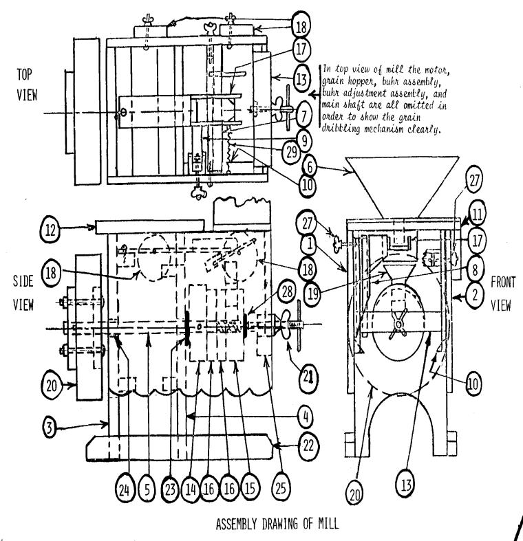
Use 3/4" thickness pine lumber. Make the foot 1 1/2" high and 15 1/2" long. Bore 1/4" to suit matching holes in details #1 and #2.
