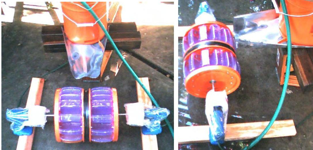
Summary: Cordless drills can be converted to generate a small amount of electricity in emergency. If hand cranked expect about 2 watts. If water powered could be tuned up to produce about 4 watts charging one cell. How long will the plastic gears last in continuous operation? This is anyone's guess. I think with regular maintenance of opening the gear box and relubricating that it may last a time. However, at about \$10 per generator one could stock up on a few extras.
