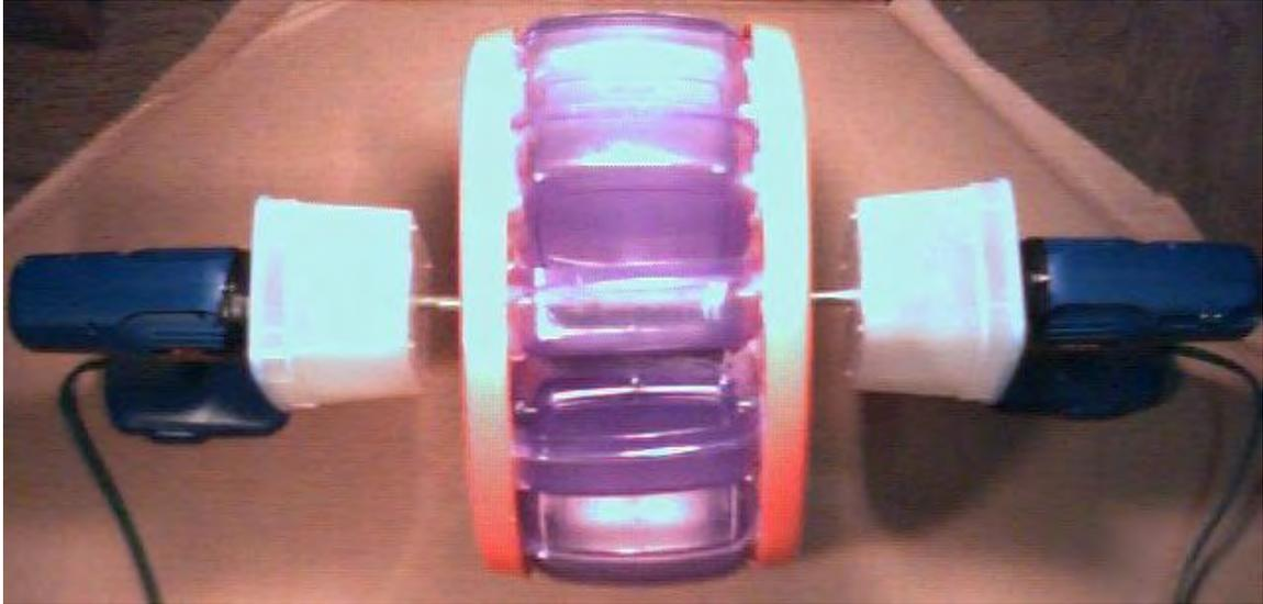
Stack one at a time plastic container on top and nested in the lower one. Then drill in a hole in the middle of one of the longer sides. Use a #8-32 by .5" long machine screw and nut to fasten them together. The containers are positioned so the overlap is just enough to bolt them together. See <http://home1.gte.net/mikelob/WaterW-1.JPG>
