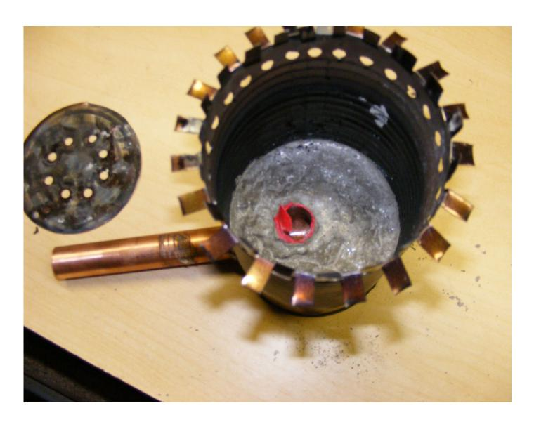
This is what it looks like down inside the burner. Tape is still ther but will be removed as it was used to cover the hole so no concrete would get inside.
