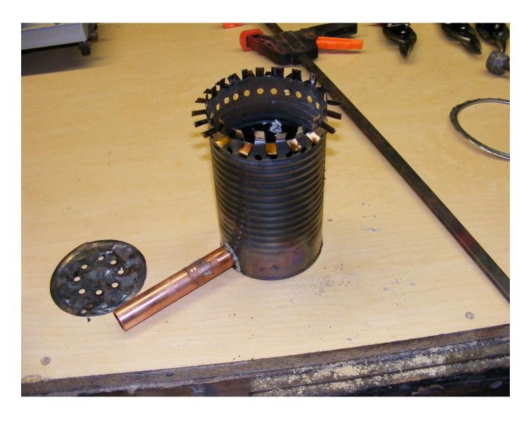
This is a picture of the burner after the concrete set up. The pipe will go through the secondary air can and the outside 5 gallon bucket.
