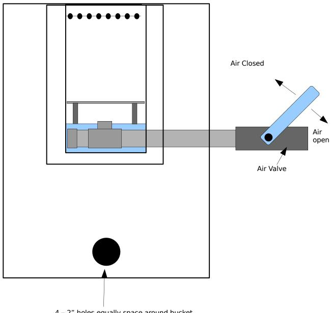
4 – 2" holes equally space around bucket This is to allow secondary air in
