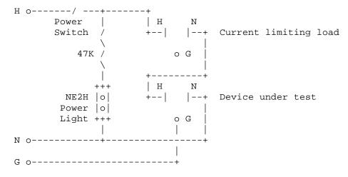
Note: Ground connections normally not used for equipment likely to be tested using this device.
