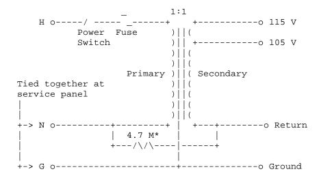
Note: Ground is included on the secondary side. This is actually needed for safety with certain types of equipment like microwave ovens where the HV return is to the chassis. Most other consumer electronics equipment and appliances will only have a 2 wire cord and thus not use the Ground.
