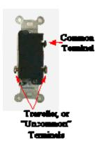
The heart of a 3-way circuit is the 3-way switch. Unlike a common wall switch, the 3-way switch has three active terminals (plus a ground in up-to-date installations). Only one of them is important to identify for the purposes of replacement... the **common TERMINAL**. Though our graphic (left) shows the common terminal in a certain position, the fact is that it could be any terminal on your individual switch.
