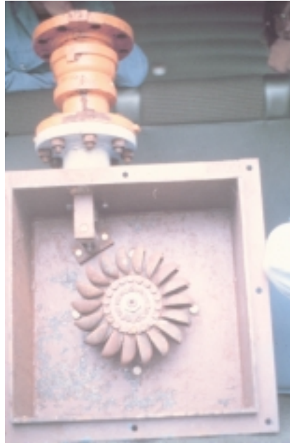
Even seasonal streams will supply power in the winter from units like this pelton wheel.
