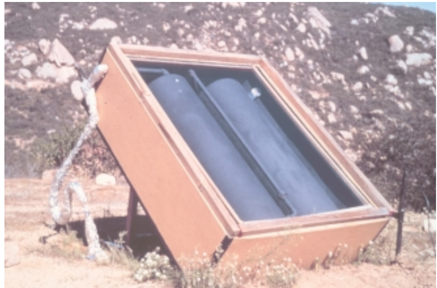
This design of solar water heater exposes the tanks directly to the sun in an insulated box.
