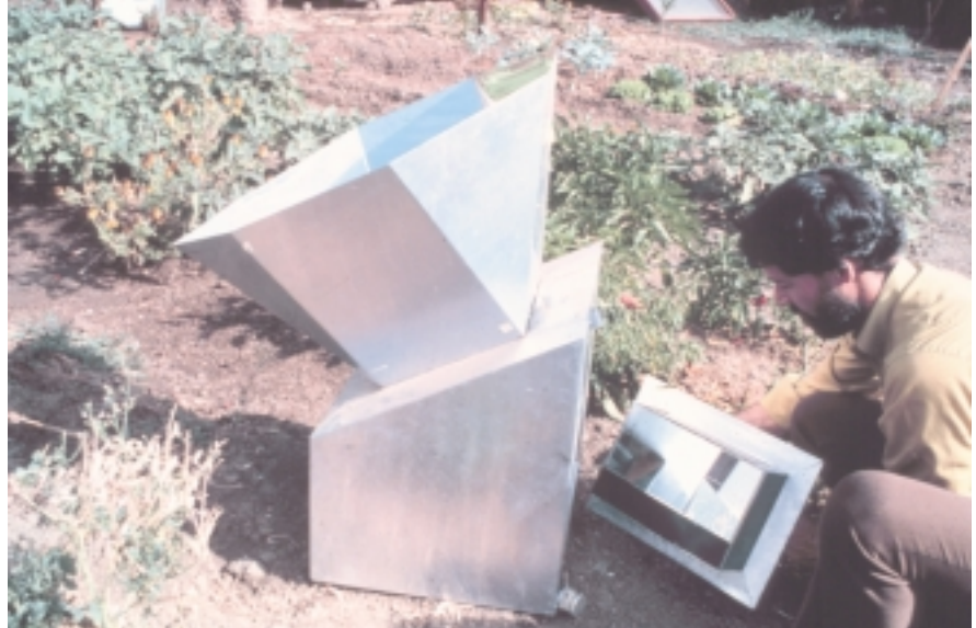
Solar cookers achieve 250-350 degrees during operation.
