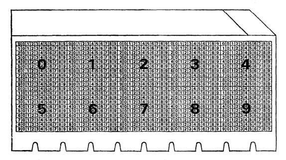
FIG. 3. Diagram of a 1,000-position peek-a-boo card.
