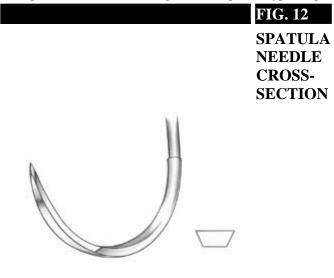
The SABRELOC spatula needle has two cutting edges and a trapezoidal-shaped body.
