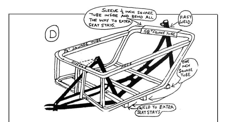
don't be afraid to flatten the stay a little - bike tubing is very strong. However this should not be necessary.
