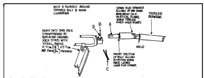
Hole A is slipped over tapered bolt B, then split pin C is inserted through hole D. Split pin holds trailer coupling on towbar, and provides easy 'no tools' quick release of trailer, Split
