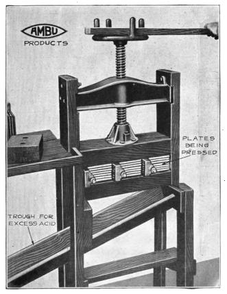
Fig. 77. Battery Plate Press
