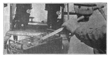
Fig. 155. Chiseling Off Rough Edges from Tops of Posts Before Burning In
