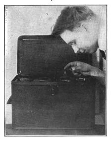
Fig. 20. Examining the Inside of Battery Through the Vent Hole in Top to See the Height of Solution
