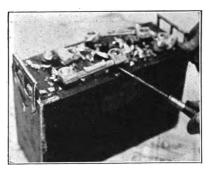
Fig. 98. Prying off Connectors with Screw Driver
