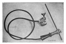
Fig. 84. Carbon Lead Burning Outfit
