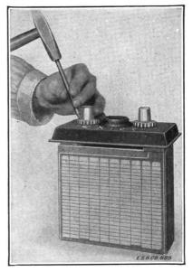
Fig. 179. Locking Sealing Nut
