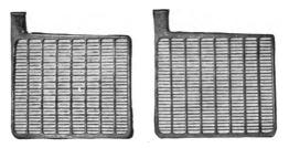
Fig. 37. A Pair of Grids Trimmed and Ready to be Pasted. The Lugs at the Top Are for Burning in to the Connector Straps to Make a Group
