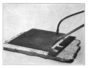
Fig. 135. Extending Lug on Plate
