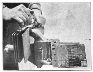
Fig. 133. Sawing Slot in Plate Connecting Strap
