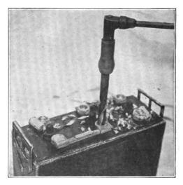
Fig. 97. Drilling Posts and Top Connectors Digitized by GOOgle
