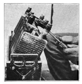
Fig. 112. Taking Off Covers with Two Screw Drivers
