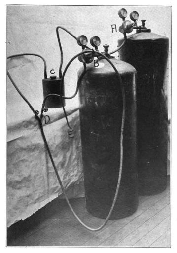
Fig. 85. Hydrogen-Oxygen Lead Burning Outfit. A and B are Regulating Valves. C is the Safety Flash Back Tank. D is the Mixing Valve. E is the Burning Tip (c) The Prestolite Company of Indianapolis sells a lead burning outfit which uses Prestolite gas and oxygen under pressure.
