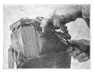
Fig. 166. Removing Covers from Willard Type S Battery Digitized by GOOgle
