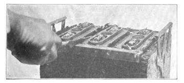
Fig. 164. Removing Pitch with a 1/3 -inch Chisel from Covers on Willard Type S Battery Digitized by Google
