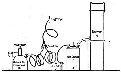
Fig. 86. Hydrogen Generating Outfit
