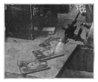
Fig. 143. Heating Lower Covers Before Replacing on Battery
