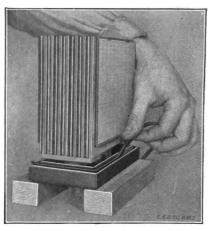
Fig. 180. Sealing Double Flange Cover
