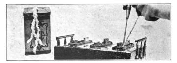
Fig. 168. Putting Asbestos Packing Around Post in Willard Type S Battery, to Prevent Compound from Running Down Into Cell When Burning In
