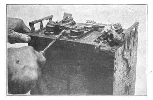
Fig. 163. Removing Top Connectors with Screwdriver. Note Angle Iron Held on Edge of Case to Prevent Damaging Case. Willard Type S Battery
