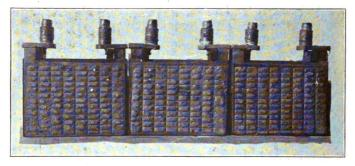
Fig. 124. Badly Bulged Negatives. Such Plates Need Pressing
