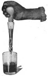
Fig. 24. Release the Pressure on the Bulb, Thus Drawing Water Up Into the Hydrometer
