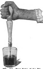
Ffg. 23. Pour Some of the Distilled Water Into a Glass. Squeeze the Air Out of the Bulb of the Hydrometer. Put Rubber Tip in the Glass
