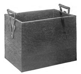
Fig. 49. Battery Box or Case with Handles. It Is Made from Kiln-Dried Oak Lumber and Thickly Coated with Acid-Proof Paint. All Metal Parts, Other Than Lead. Are Lead-Coated to Keep Them from Corrosion by the Acid in the Battery Solution
