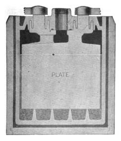
Fig. 29. Showing Battery with Electrolyte too Low
