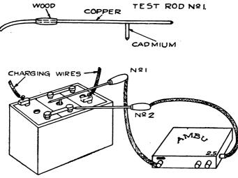
Fig. 183. Making a Cadmium Test
