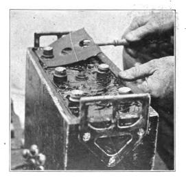
Fig. 106. Removing Top Covers with Screw Driver Resting on Angle-Iron
