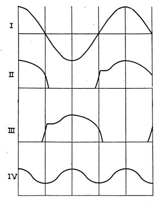
Fig. 66. Wave Form of Mercury Arc Rectifier
