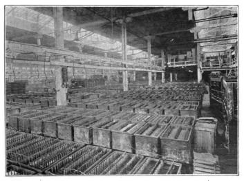
Fig. 41. Forming Room in the Willard Storage Battery Co. Factory
