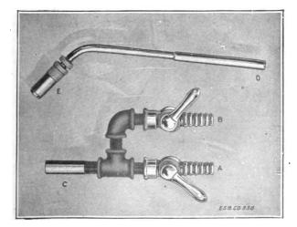
Fig. 88. Illuminating Gas Valve and  $\text{Burning}_{\text{Digitized by}} Goog[e]$
