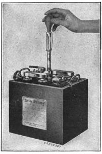
Fig. 33. Taking a Specific Gravity Reading
