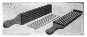
Fig. 80. Burning Lead Molds, Showing Lead Made in Them.
