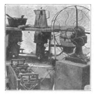
Fig. 146. Cooling Hot Compound with Electric Fan
