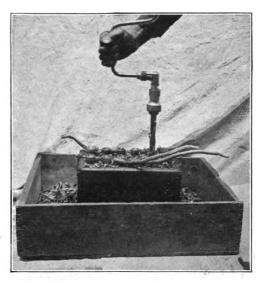
Fig. 96. Drilling Posts and Top Connectors, with Battery in Special Box
