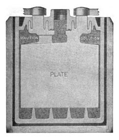
Fig. 28. Showing Battery with Electrolyte too High
