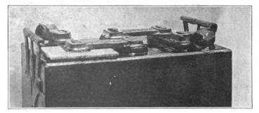
Fig. 172. Transite Board Around Cover to Protect It When Burning In Connectors
