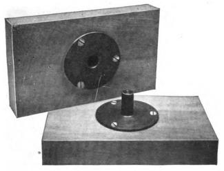
Fig. 78. Battery Turntable
