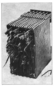
Fig. 126. Rotted Separators
