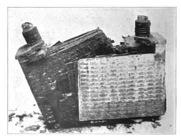
Fig. 120. Corroded, Bulged and Subhated Negatives. Disintegrated, Rotted Positives
