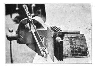
Fig. 134. Slotted Saw, a group with two Plates removed, and Slots in Connecting Strap for New Plates
