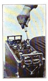
Fig. 109. Removing Compound from Edge of Case and Tops of Jars with Hot Screw Driver
