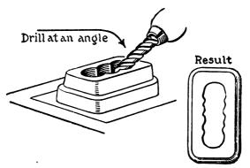
Fig. 162. Widening the Slot
