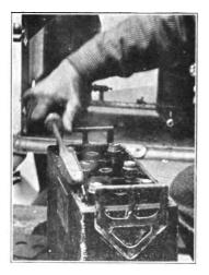
Fig. 145. Using Very Hot Sealing Iron Around Case
