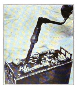
Fig. 100. Straightening Hole Which was Started Off Center
