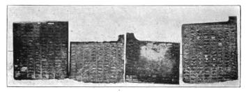
Fig. 116. Diseased Negatives. The Large Ones only Eight Months Old. Active Material Blistered, Soft, and Granulated
