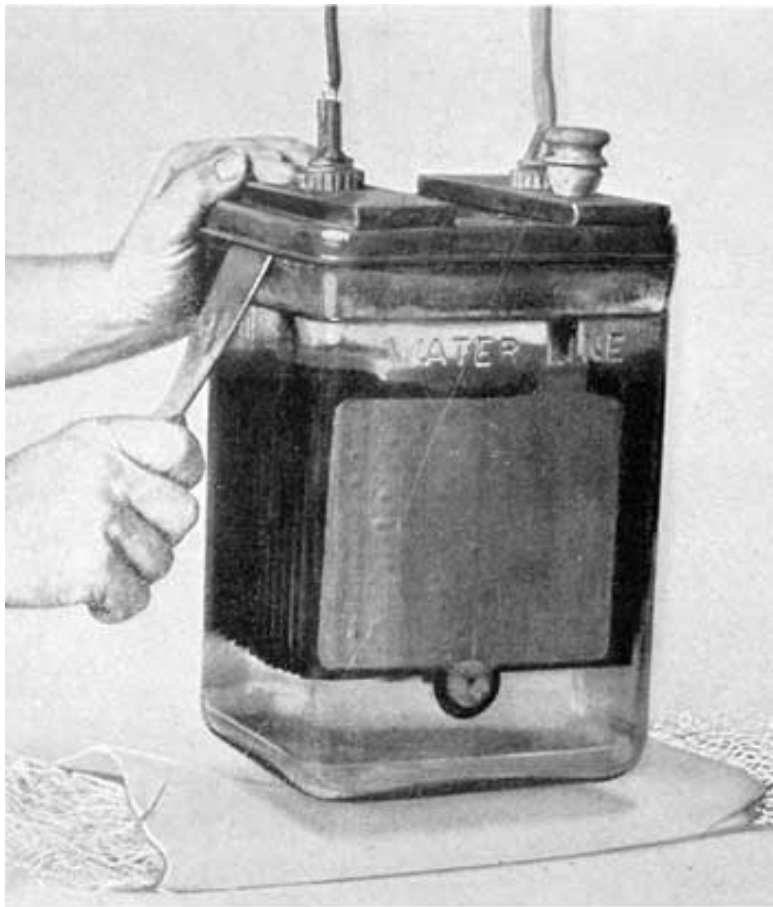
Fig. 306. Removing Delco-Light Cell Cover
