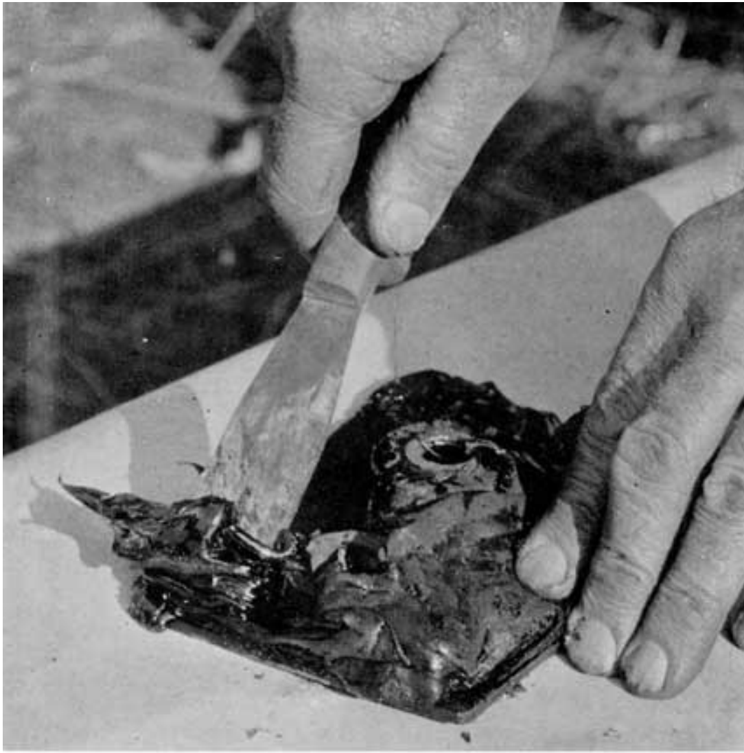
Fig. 199. Removing Sealing Compound from Double Cover
