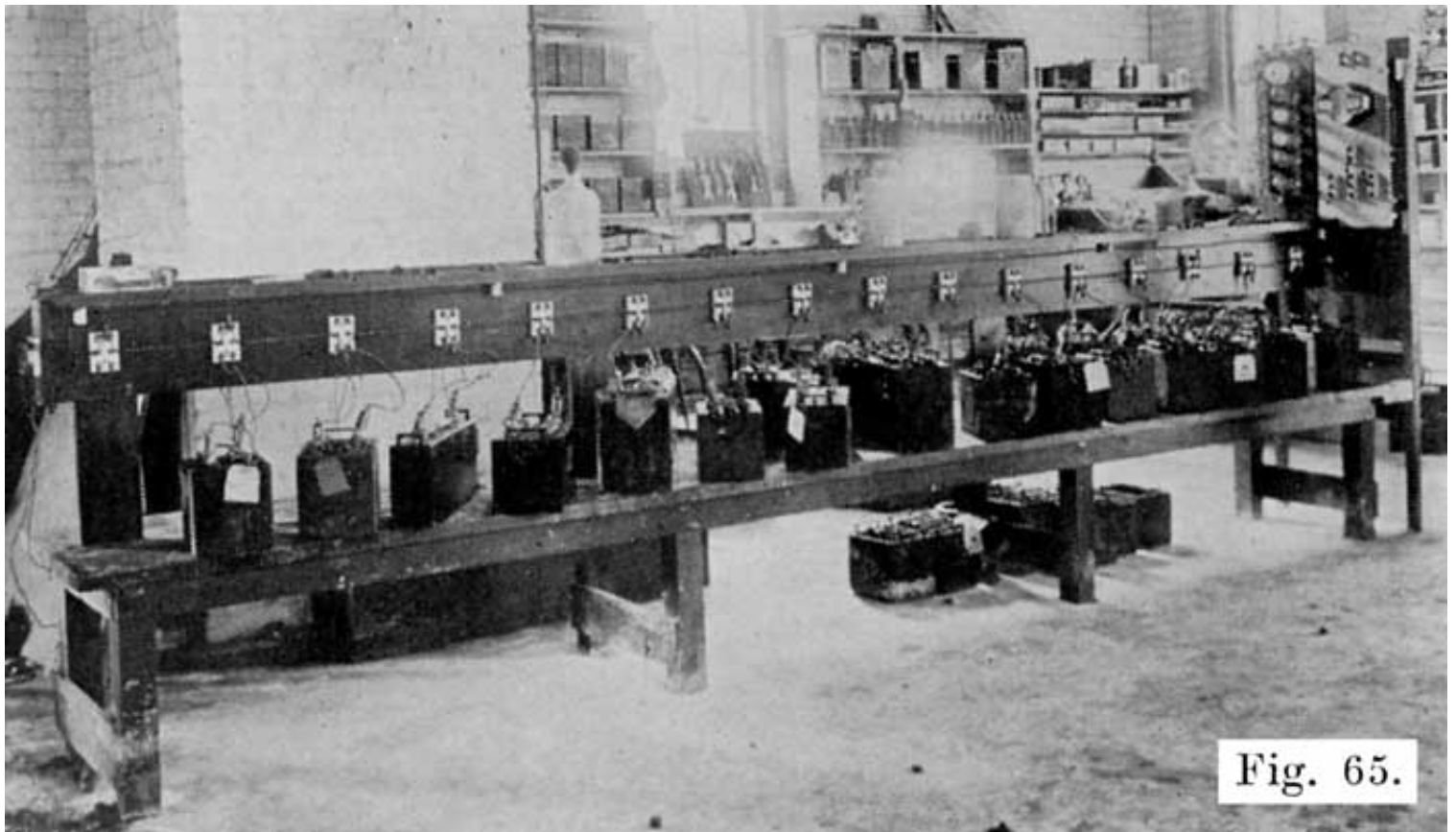
Fig. 65. Charging Bench with D.P.D.T. Switch for Each Battery
