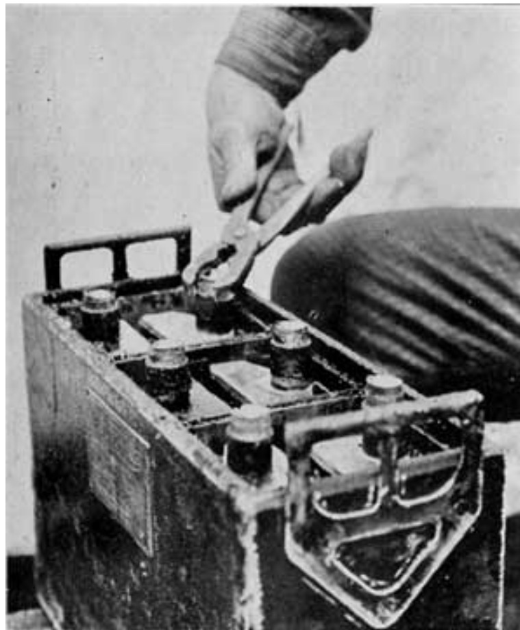
Fig. 217. Cleaning Scale From Posts Before Replacing Connectors Temporarily for Charge
