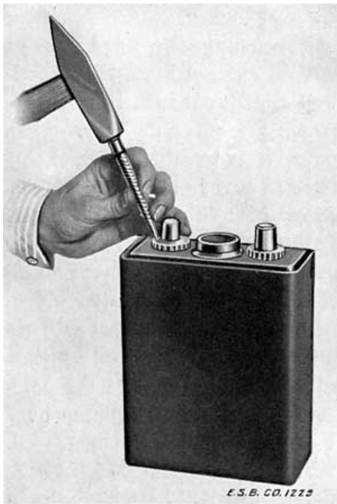
Fig. 241. Upsetting Threads to Prevent Nut from Turning
