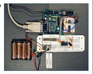
IR site would come to a standstill.) My solution was to cobble together a little MSD (Mad Scientist's Device) battery discharge tester, using a Basic Stamp microcontroller, a Linear Tech A/D chip, a relay to connect or disconnect the batteries from the load, a couple of big power resistors (to serve as the load itself), and a few other components. The whole mess is as appears at right.
