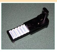
Because of their low internal resistance, Eneloops are also ideal for high-current devices. This is the battery pack for my Nikon Coolpix 8700 digital camera.
