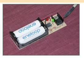
Eneloop cells can be charged in any standard Nickel Metal Hydride (NiMH) charger, including this do-ityourself USB-powered one.
